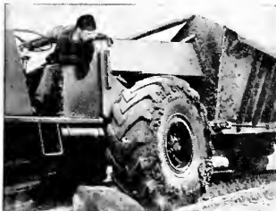
Nylon cords give giant truck and airplane tires the strength and elasticity to absorb tremendous impact shock without bruising.
