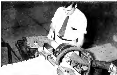
MECHANICAL ENGINEERS design equipment like this automatic vacuum "pickup" to improve methods of handling Ivory, and other soaps.
