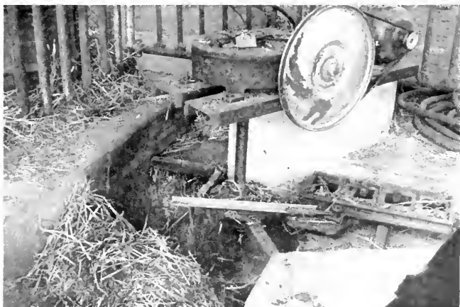
The driving mechanism of the gutter drag line.
