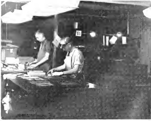
In the basement of Illini Hall. Left: Two printers, Ralph Broderick and Clyde Hall assemble the body type, headlines, and cuts into page farms. Right: The printing press in action, operated by Leo Klackner. At this stage, the magazine is near completion. After the press run the sheets are cut and bound into magazine form and are then ready to be mailed.
