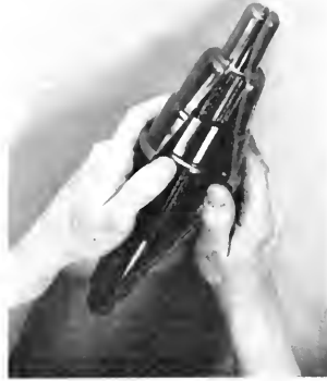
The coating can easily be removed by slitting and stripping the part.
