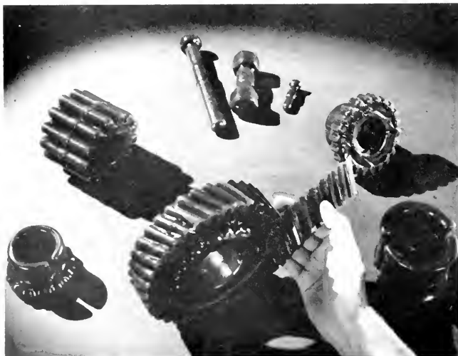
A wartime packaging development is the use of certain resins to preserve and protect metal parts in storage or shipment.
