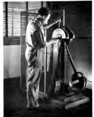
A steel sample is being given an impact test in the laboratory.
