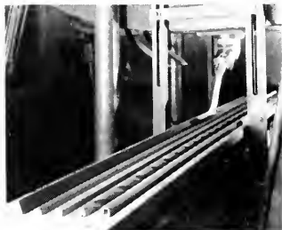
Photo showing the different shapes of cemented carbide parts produced by extrusion
