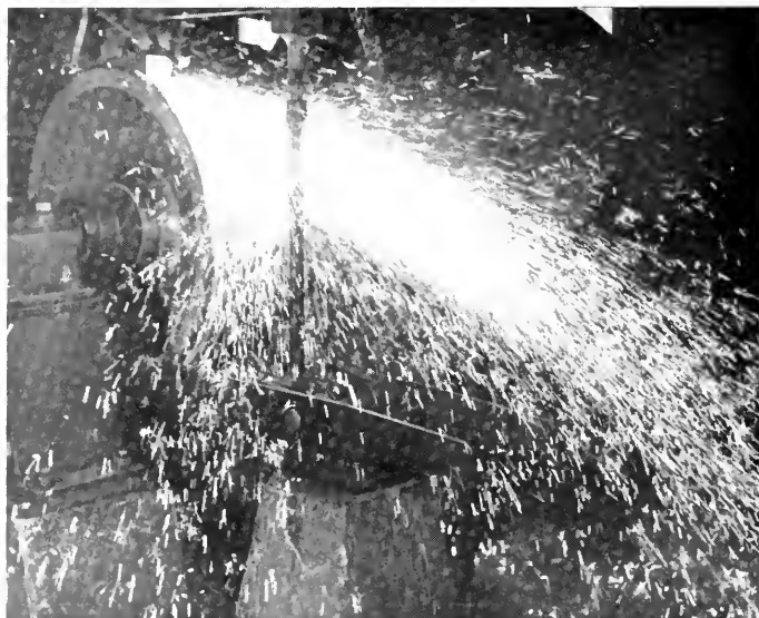
Sparks fly as this wheel "grinds" to a halt during a laboratory test simulating conditions met in stopping a fast-moving train.
