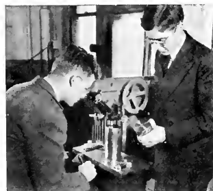
R. C. Reidinger, B.S.Ch.E., Princeton '47, and T. D. McKinley, B.S.Ch., Worcester Polytechnic Institute '35, making a test of the hardness of ingots of Du Pont titanium metal.
