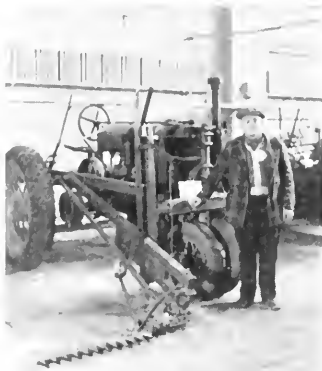
This device made with old parts and ingenuity, trims weeds close to fences.
