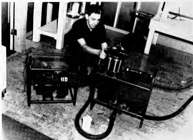
Mr. Bowman of the Sanitary Engineering laboratory displays a model of the 15 g.p.m. diatomite filter pack unit developed by the Army.
