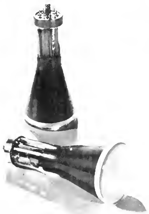
This 6-inch long cathode ray tube is designed for small, lightweight equipments.
