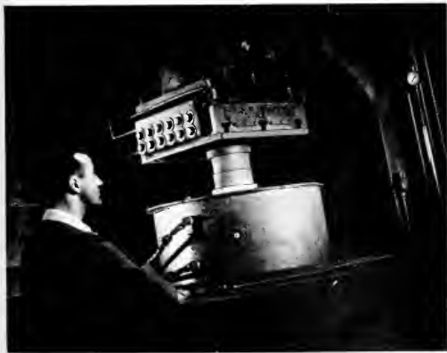
Left: Formation of carbide parts by hot pressing, a single operation which combines the three distinct processes of pressing, pre-sintering, and sintering. Right: A chart showing the relative hardness of three common tool materials as a function of temperature
