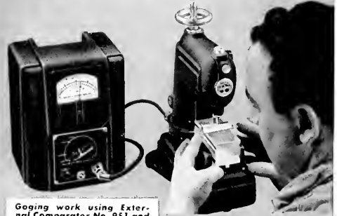
Gaging work using External Comparator No. 951 and Amplifier No. 950.
