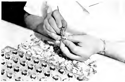
Assembling miniature electron tubes—typical of the high precision work at Allentown—calls for finest lighting. It is provided by a scientifically designed system containing over 13,000 fluorescent tubes.
