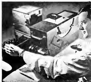
Mark P. Morse, B. S., Physics, Washington College '40, measures specular and diffused reflection of a sample paint surface with a goniophotometer, a Du Pont development for obtaining data on gloss and brightness.
