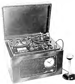
Tape recorders can be equipped with sound-activated start-stop mechanisms.
