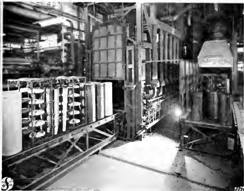
Left: Heat treating furnace used for sealing glass liners to the metal case. Right: View of the overhead conveyor system for moving parts through the plant
