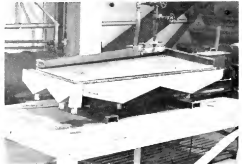
Left: Flotation separator used to segregate ore by agitation. Right: Wilfley shaker table used for gravitational separation of ores
