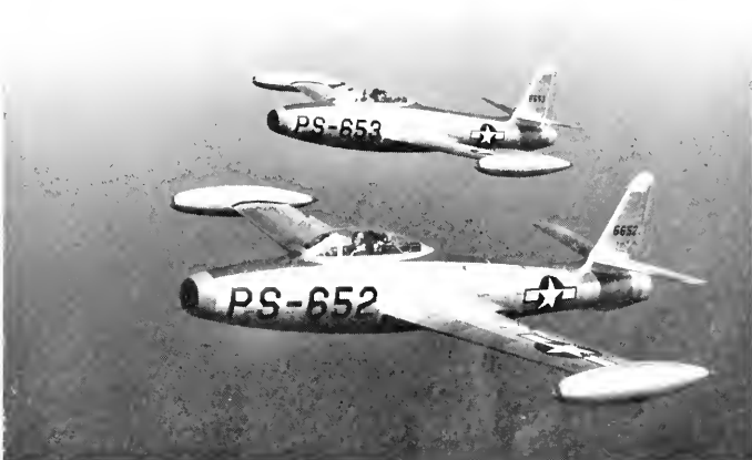
Wing tanks give the Republic P-84 Thunderjet a range of over 1000 miles. (Photo Courtesy of Flying.)
