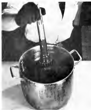
First operation of double dipping process is to immerse half of the part.
