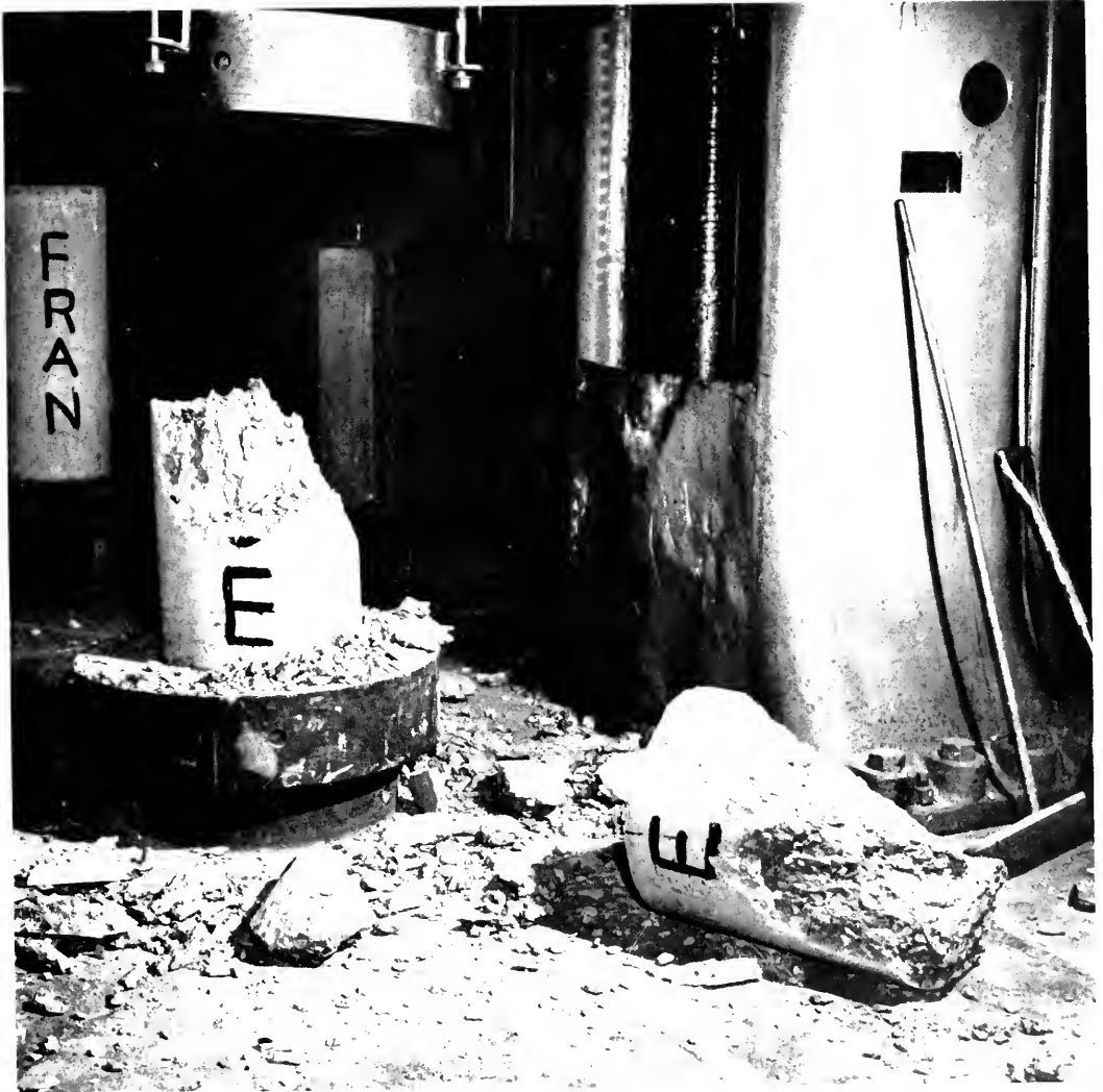
This concrete cylinder has just been shattered by the 3 million pound testing machine whose base is shown at the right.
