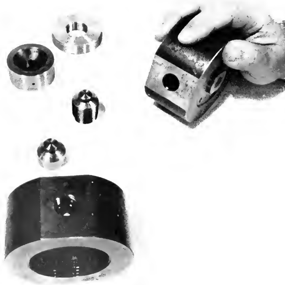
This bomb is used to obtain extremely high pressures. Variations in pressure are detected by the defraction of light rays passing through the high pressure area.
