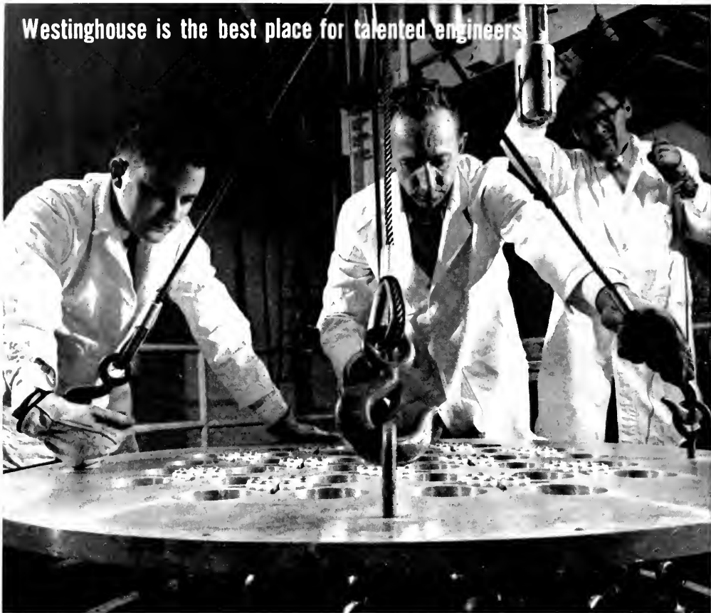
F. Kelly, W. J. Miller, and J. P. Tobin of the Westinghouse Atomic Power Department lift the "core plate" off the nuclear core for the first U.S.-built power reactor designed for use abroad (Mol, Belgium).
