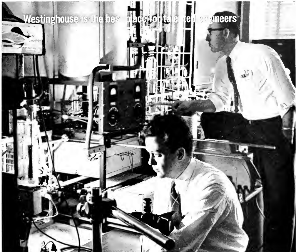
Westinghouse Metallurgists, Dr. M. J. Fraser (foreground) and Dr. H. W. Weart, prepare to photograph a molten alloy sample as one step in the determination of liquid-solid interfacial energy. These direct experimental measurements are the first of their kind ever attempted.
