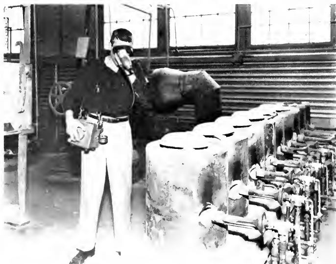
Determining the temperature of a porcelain enamel smelting furnace by means of an optical pyrometer.
