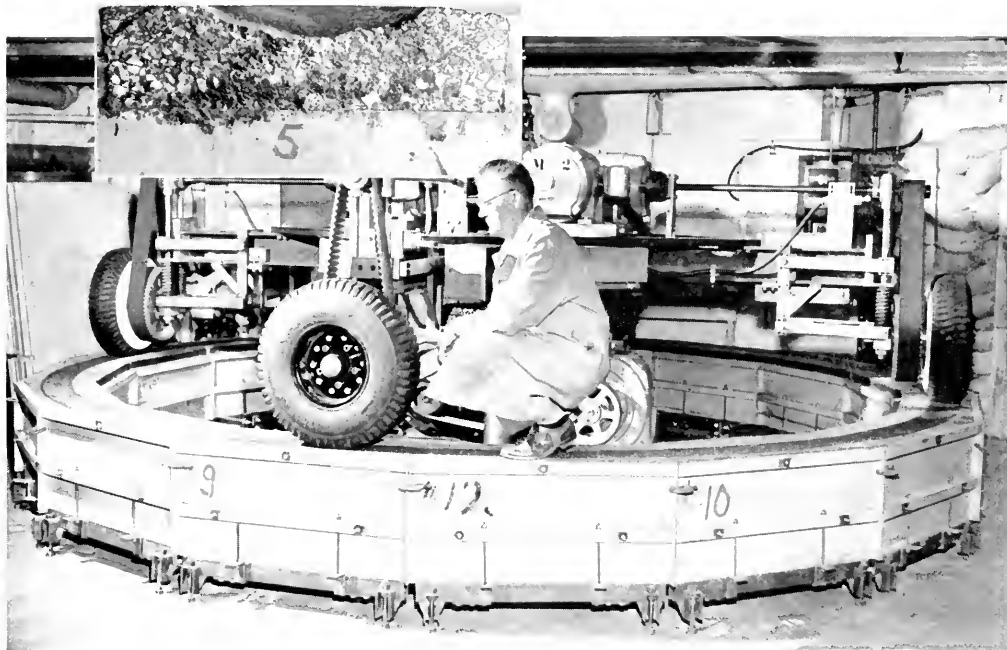
Tom Speer , Senior Engineering Research Supervisor at Standard Oil, inspects one of the 12 sections in a new miniature road tester. Under simulated weather conditions, four wheels
