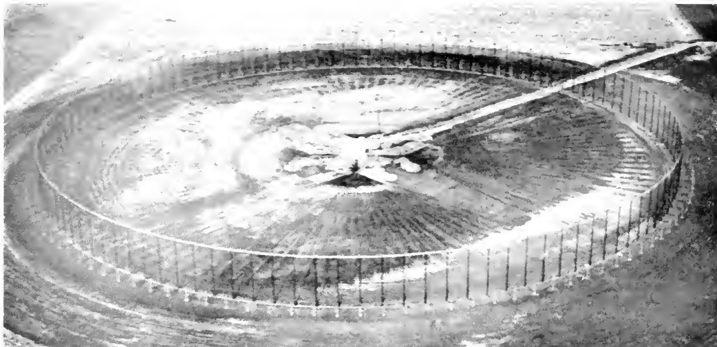
Fig. 2. The advantages of a wide-aperture direction-of-propagation measuring device are studied by radio direction finding researchers with this Wullenweber system, which has a diameter of 1000 feet.
