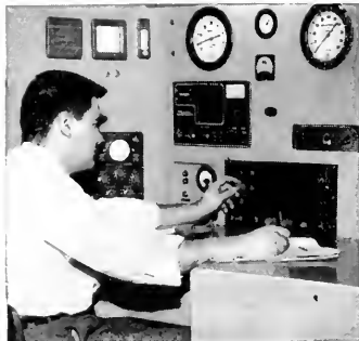
FATIGUE SPIN RIG uses compressed air to drive balls around the bore of a test cylinder to determine cylinder's static fatigue life.
