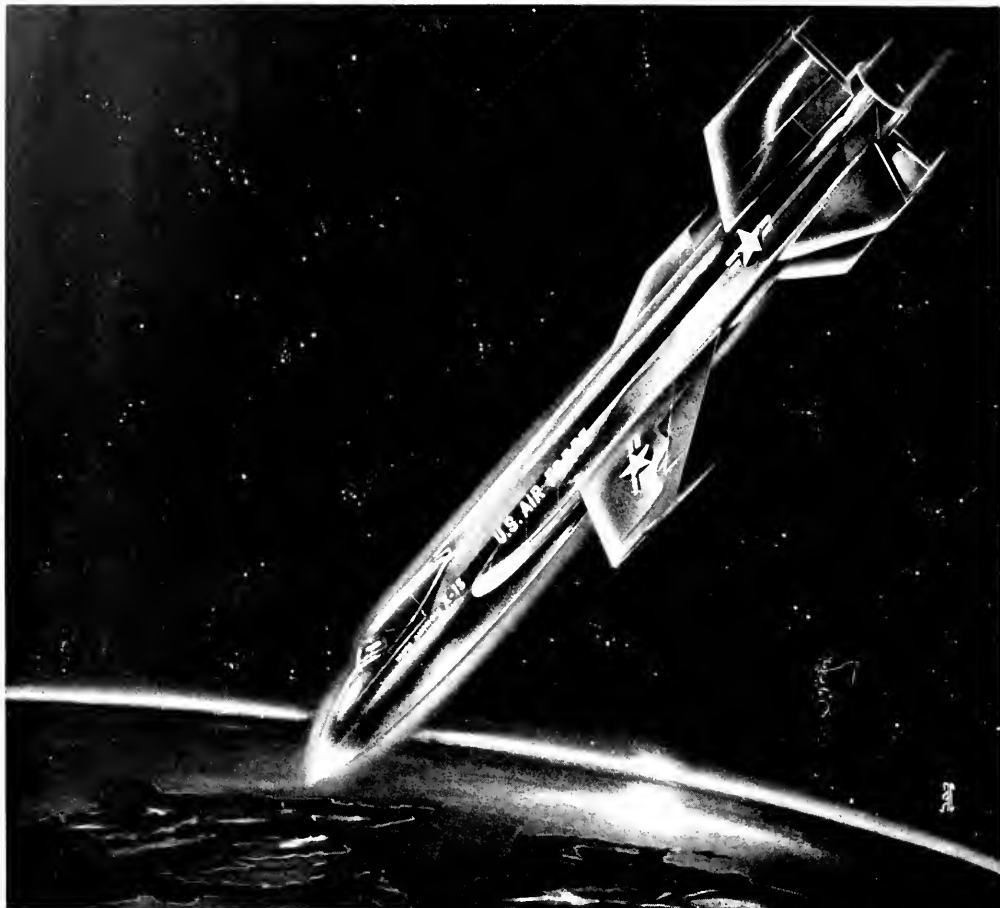
Nosing its way down to earth, X-15's skin of a high-Nickel-containing alloy will glow with the dull cherry red of a tossed rivet.
