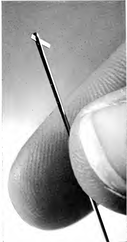
Needle's eye holds electronic "brain" cells — Photograph shows how new RCA "logic" element can be contained in the eye of a sewing needle.
