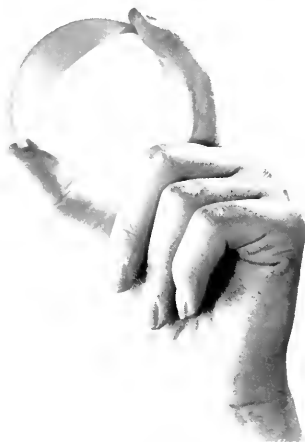
Irtan optical material finds job as nose cone for heat-seeking missiles.
