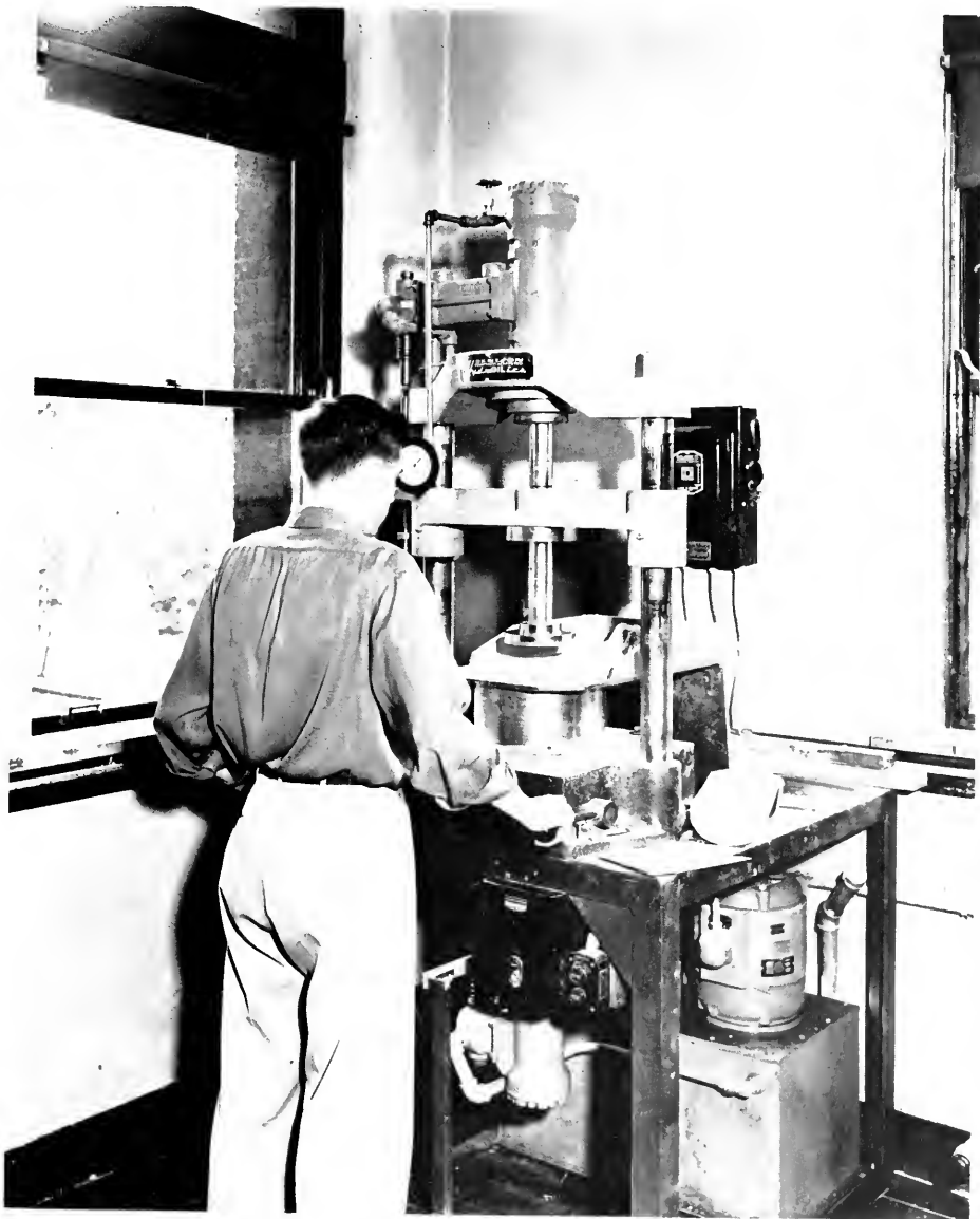
An hydraulic press is used to form dry shapes of ceramic materials in a study of desirable dies and pressure relationships.
