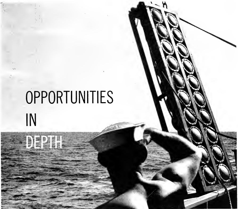
The device about to be submerged is an "underwater sound source". It transmits sound waves beneath the sea and is part of the research equipment developed by Bendix Research Laboratories Division for use in the Bendix program of undersea acoustics research.
