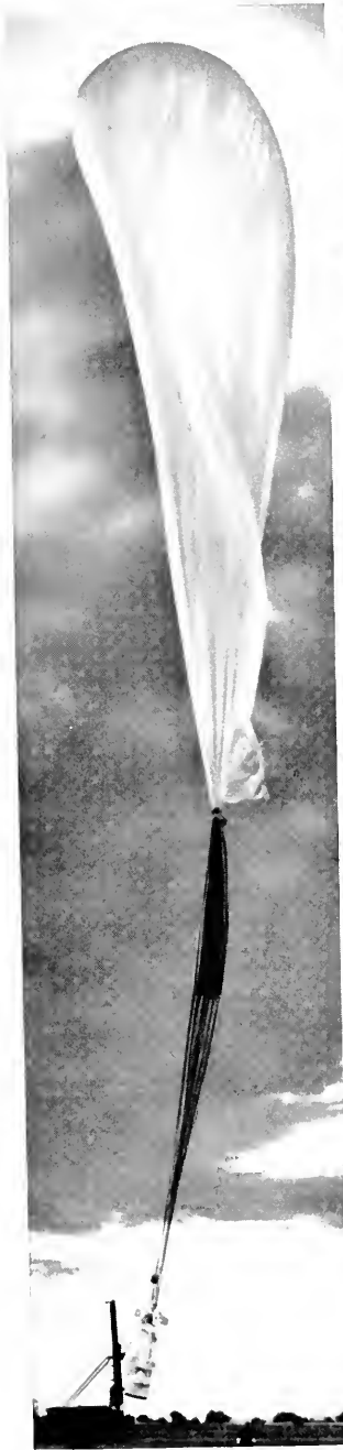
Going up for "good seeing." Unmanned balloon-observatory starts its ascent to take sunspot photos. "Project Stratoscope" is a continuing program of the Office of Naval Research and the National Science Foundation.
