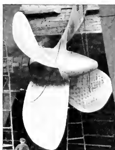
Ship's propeller—Needed: lighter weight and resistance to erosion and salt water corrosion. Which alloy... ?
