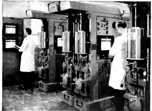
Creep-Stress Rupture Laboratory in our new Steel Research Center. Here we test the resistance of steels to deformation at temperatures as high as 1800° F.
