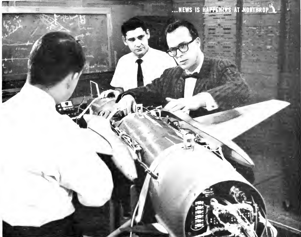
Engineer Larry Klivans reviews the results of a computer-simulated ground checkout of Radioplane Division's near-sonic RP-76 rocket-powered target drone. Formerly
