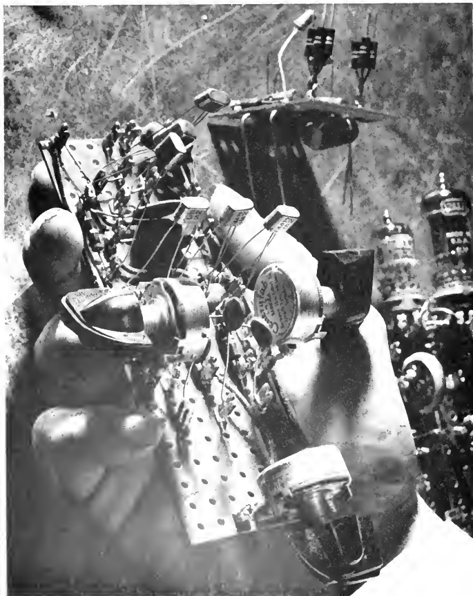
This electronic package is an artificial neuron used in a biological computer
