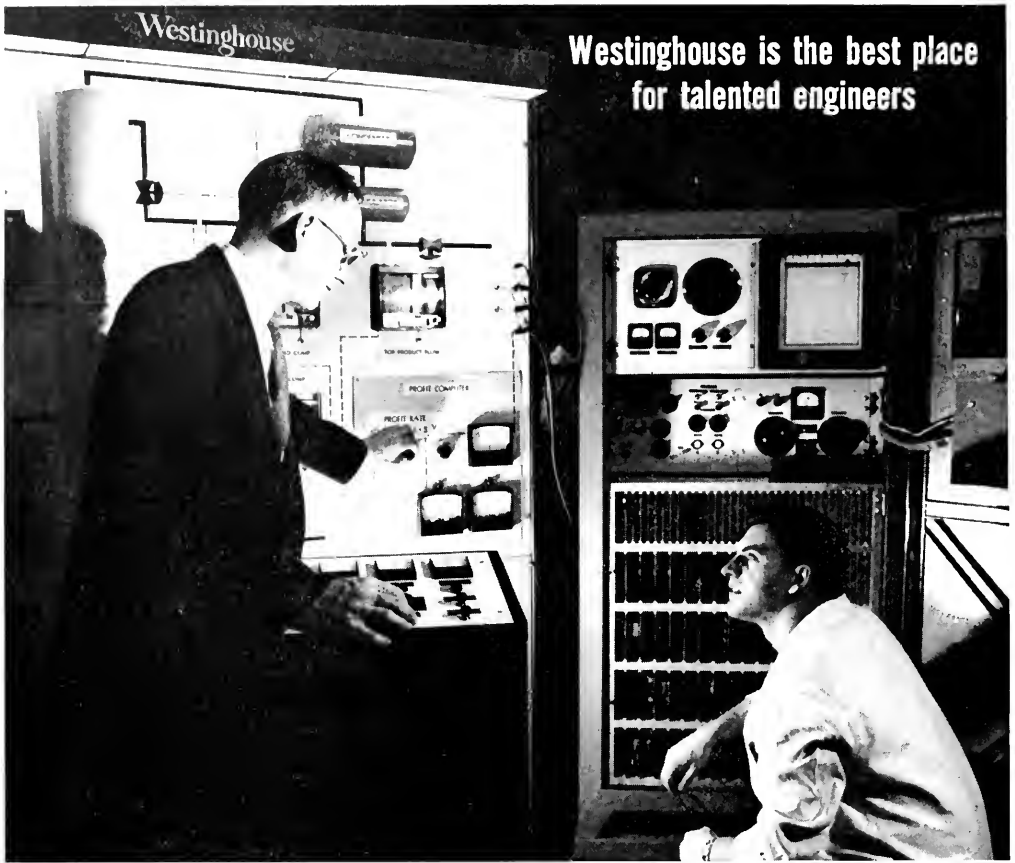
Engineer C. A. Booker and Technician L. G. Szarmach run an optimizing control test to achieve the highest profit rate for a simulated chemical distillation process.
