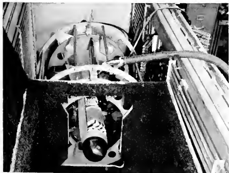
Falcon air-to-air guided missiles, shown in an environmental strato chamber are being developed and manufactured by Hughes engineers in Tucson, Arizona.
