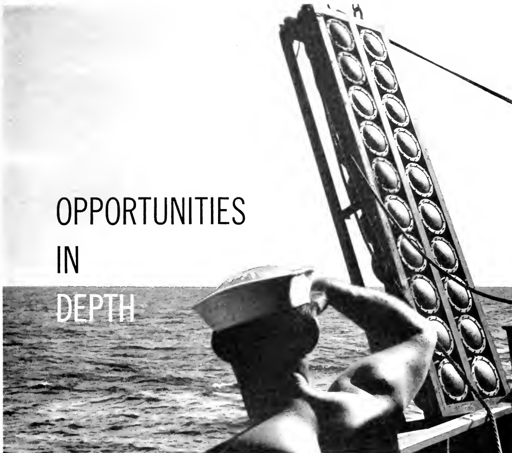
The device about to be submerged is an "underwater sound source". It transmits sound waves beneath the sea and is part of the research equipment developed by Bendix Research Laboratories Division for use in the Bendix program of undersea acoustics research.
