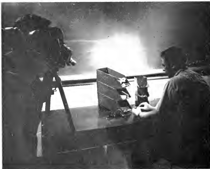
Time and motion study utilizes many modern devices to improve output and save labor. Shown here is a camera recording the procedure used in an assembly process.
