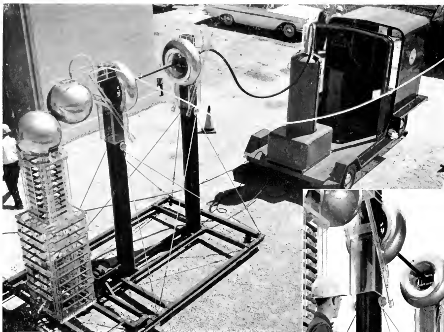
Test engineers (right) assemble high potential testing equipment. The complete installation (upper) consists of a completely enclosed electrostatic generator (on right) which has a current output of four milliamps and a voltage output of 600,000 volts. The electrostatic generator feeds into a current-limiting and discharge assembly in the lower left of the picture.
