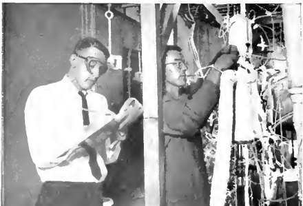
Under the close supervision of an engineer, final adjustments are made on a rig for testing on advanced liquid metal system.
