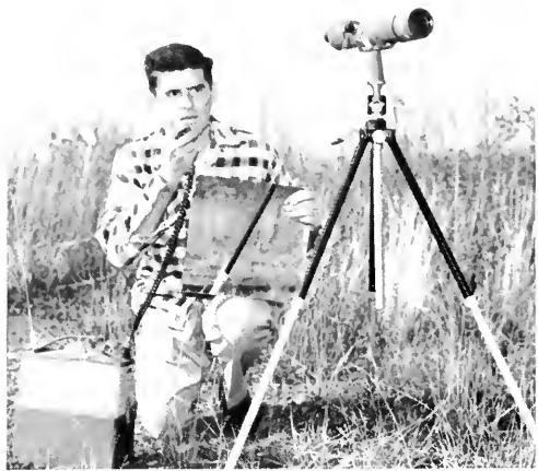
Here, Dick checks line-of-sight with a distant repeater station by mirror-flashing and confirms reception by portable radio. Using this technique, reflections of the sun's rays can be seen as far as 50 miles.
