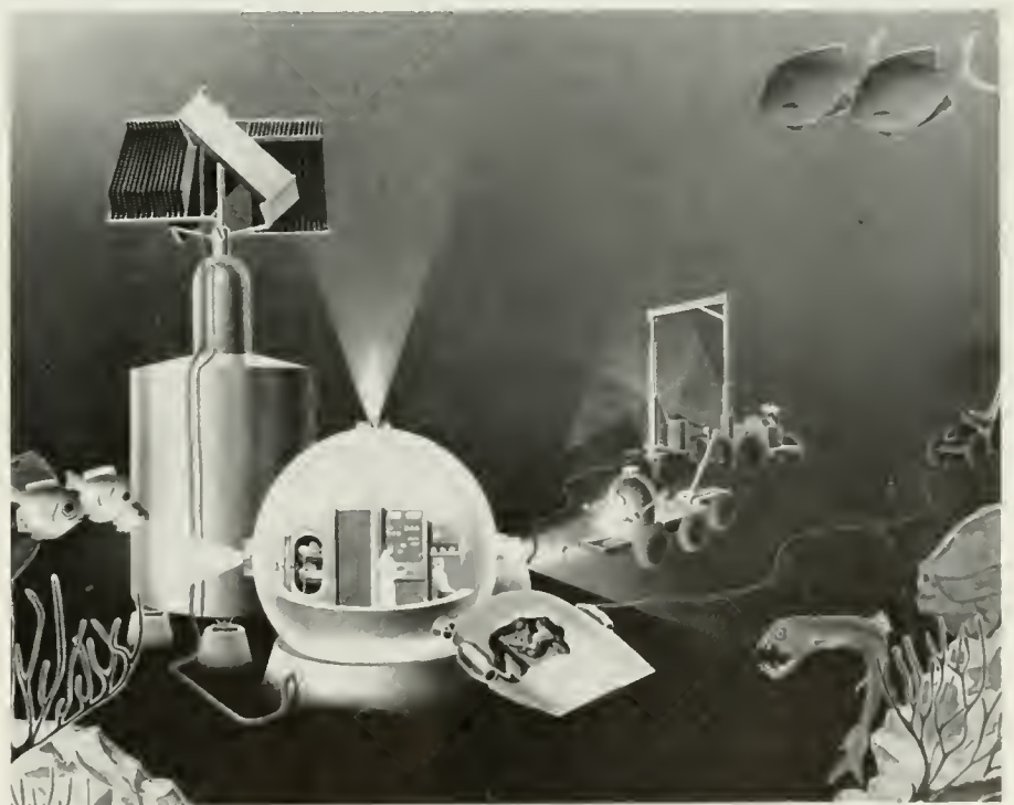
Figure 3. This artist's sketch shows how man could explore "inner space" and tap the vast natural resources on the ocean floor through the use of an advanced power generation system unveiled recently. Heart of the system is an undersea nuclear reactor (left) capable of producing 3000 kilowatts of electricity for life support and operational activities in a two-mile deep undersea community. (Photo courtesy of Westinghouse College Editorial Service.)
