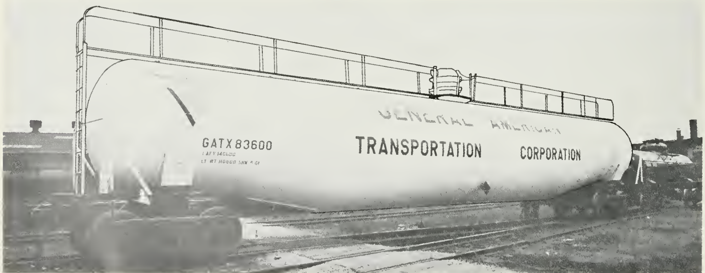
This General America Transportation Company tank car has a capacity of 30,000 gallons and is about twice as long as the old tank cars.
