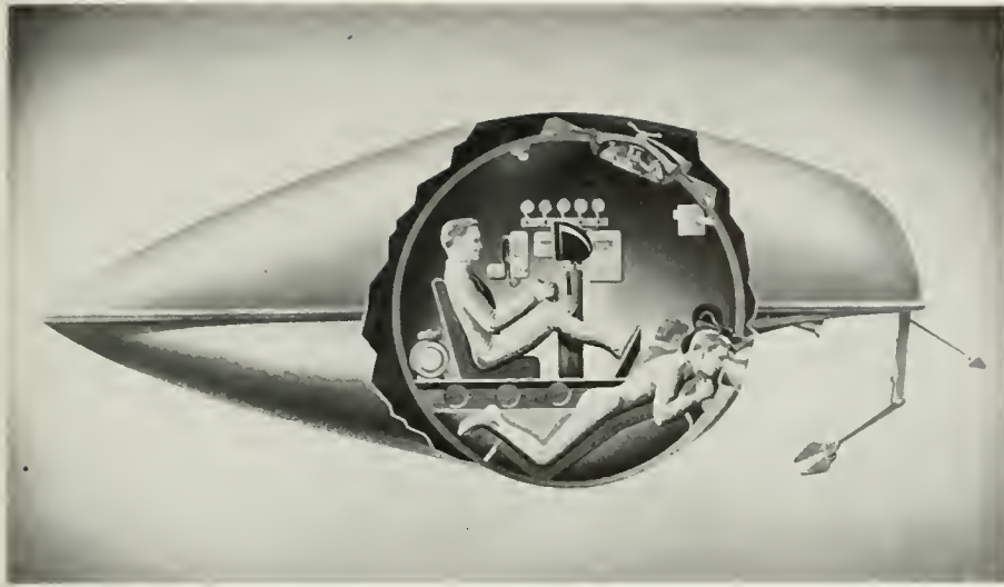
Figure 2. The "Deepstar," a three-man, self-propelled deep sea vehicle, is capable of doing useful work at a depth of 12,000 feet. Equipped with remotely controlled arms for collecting samples and for lighting, the vehicle is designed to provide optimum maneuverability and versatility for research work. (Photo courtesy of Westinghouse College Editorial Service.)
