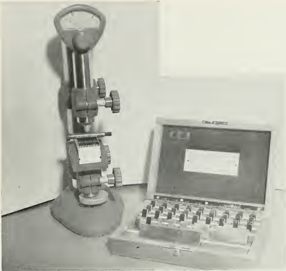
Figure 1. A Mikrokator and a set of "Joe Blocks" used in precision measuring. The blocks are guaranteed accurate to within two millionths of an inch.
