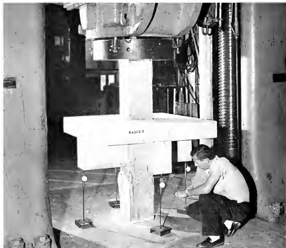
Figure 1. A graduate student is examining the failure in a reinforced concrete specimen. The specimen was loaded by the partly visible machine, which can exert 3,000,000 pounds of compression or expansion.
