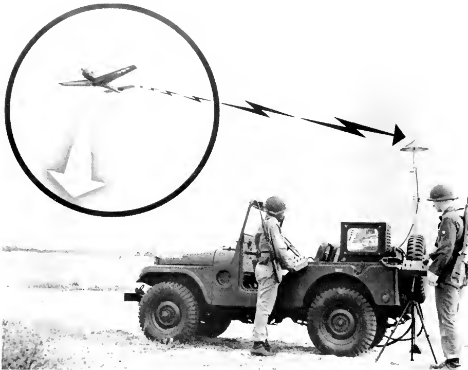
Figure 1. Unmanned aircraft send back aerial views of distant sites, using light TV equipment developed at the Army's Signal Corps Engineering Laboratories at Fort Monmouth. The camera in the L-17 drone (shown in telescopic view) can point downward or forward through the plane's belly.
