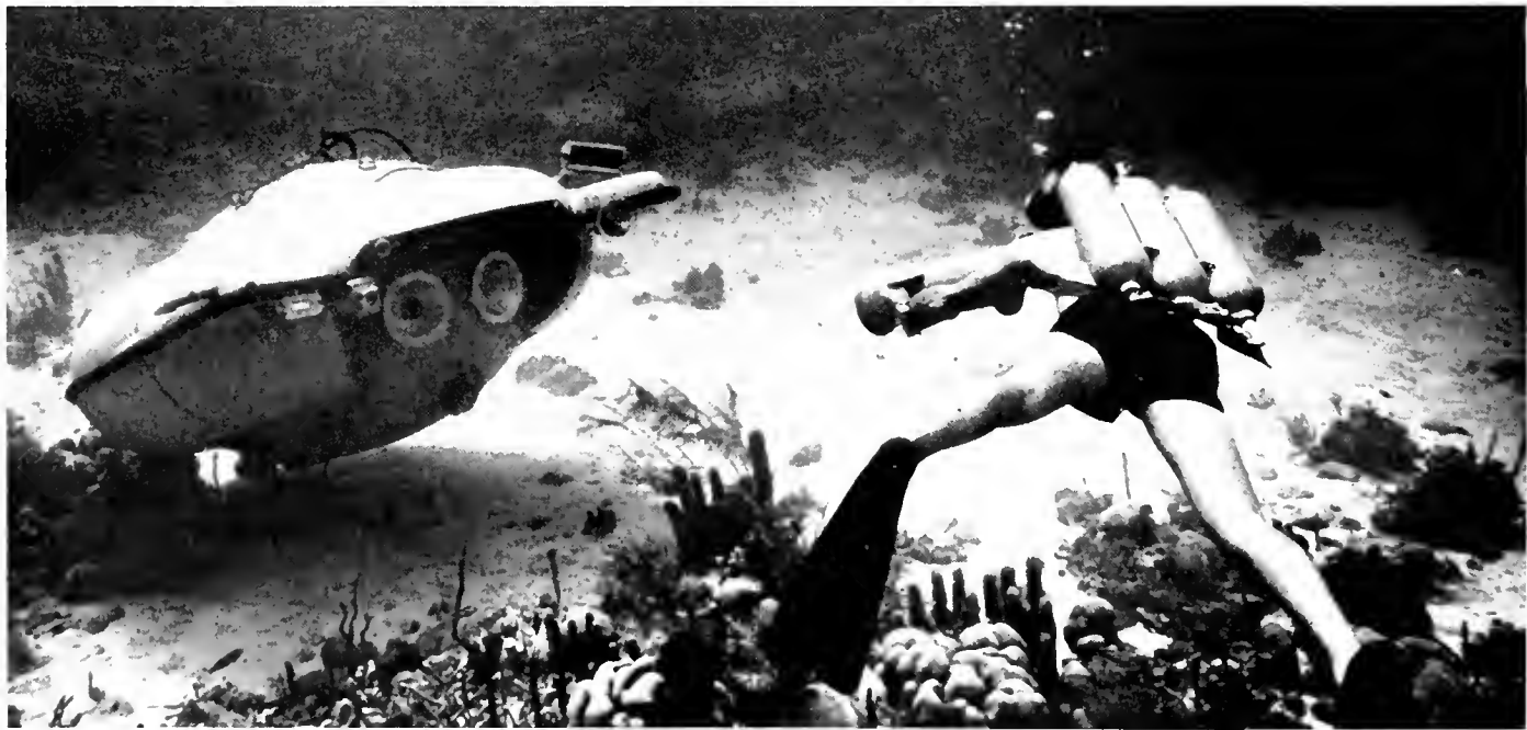
Figure 1. The "Diving Saucer," an undersea exploration vehicle, is capable of operating at a depth of 1000 feet and is the forerunner of the more advanced "Deepstar." (Photo courtesy of National Geographic Magazine and Westinghouse College Editorial Service.)
