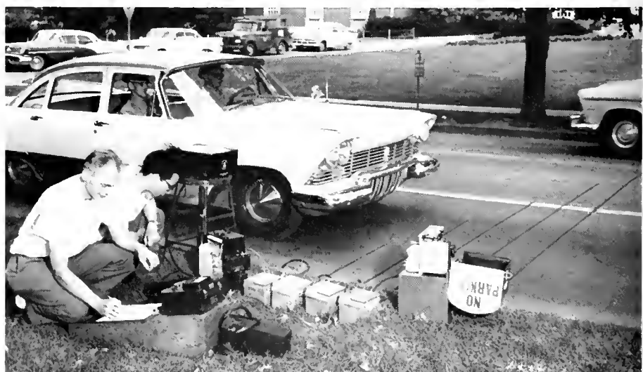
Figure 1. The speed, volume and lateral placement of vehicles traveling along this street on the University of Illinois campus are being recorded as part of a research project on traffic stream characteristics.
