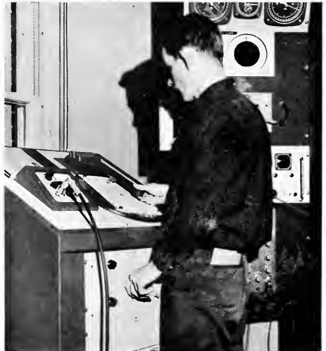
John Kimball, a junior in engineering physics and a student technician in the antenna laboratory, operates the polar pattern-recorder in the low-frequency antenna testing range.
