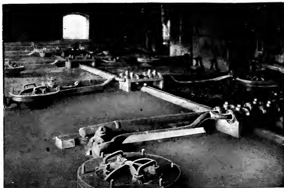
FIG. 226.—Covers of animal charcoal filters with piping.
