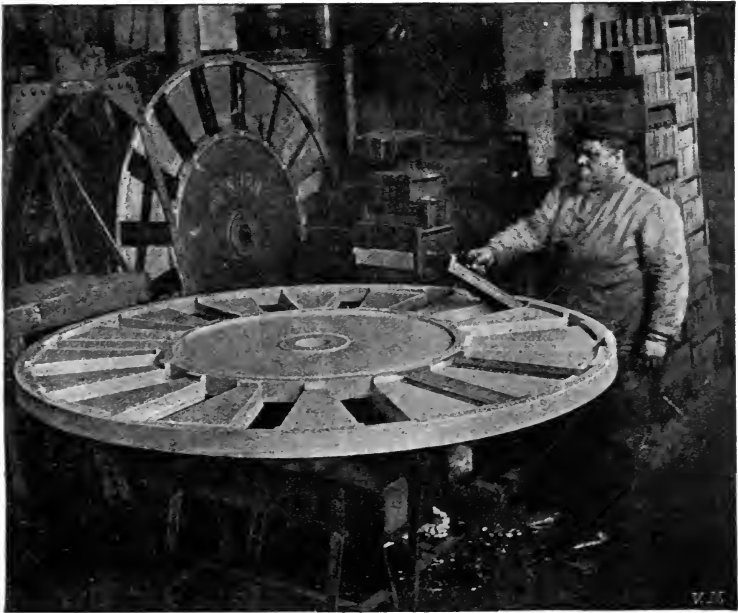
FIG. 20.—Removing knife-holders from plate of beet-slicing machine.
