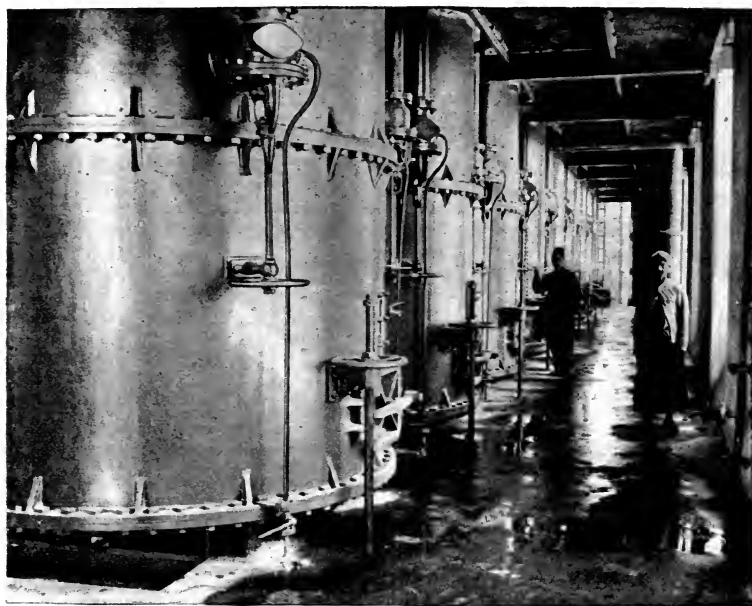
FIG. 208.—Clarifiers for cane-sugar juice, Nagi Hamadi cane-sugar factory (DANEK).
