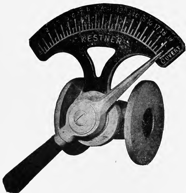
FIG. 183.—Dial water valve for use in maceration process (KESTNER).
