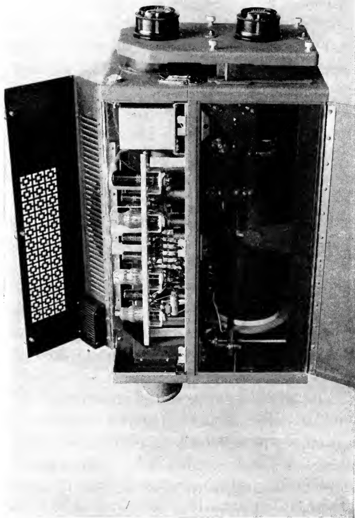
INSIDE VIEW OF STANDARD PICKUP CAMERA
