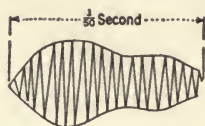
FIG. 5.—OSCILLOGRAM OF CURRENT Letter "B" 1,000-cycle tone. (Flowers. Trans. Amer. Inst. El. Eng. )
