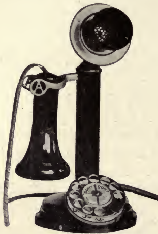
FIG. 43.—AUTOMATIC TELEPHONE STATION
