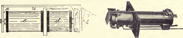
FIG. 50.—ELECTRICALLY-OPERATED SELF-RESTORED DROP
