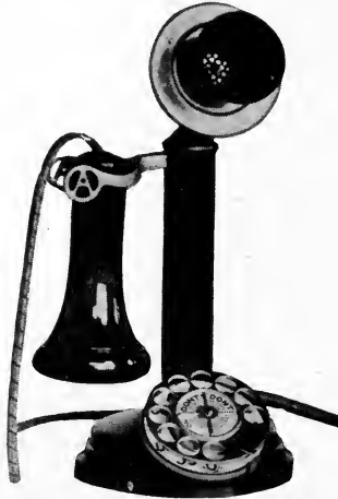
FIG. 43.—AUTOMATIC TELEPHONE STATION
