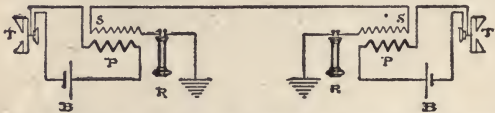
FIG. 16. DIAGRAM OF COMPLETE TELEPHONE CIRCUIT. T TRANSMITTER, B BATTERY, P PRIMARY, S SECONDARY, R RECEIVER.
