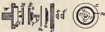
FIG. 42. DETAILS OF SOLID BACK TRANSMITTER. W ELECTRODE CHAMBER, i INSULATING LINING, B BACK ELECTRODE. a BRASS BACKING, E FRONT ELECTRODE, b BRASS BACKING, p THREAD FOR NUT U , m MICA WASHER, u NUT FOR CLAMPING m IN PLACE, p' THREAD FOR t AND t' , c COVER OF W , TT NUTS FOR CLAMPING FRONT ELECTRODE TO DIAPHRAGM
