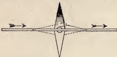
FIG. 5. ACTION OF CURRENT ON MAGNET. DOTTED LINES SHOW NORMAL POSITION OF MAGNET.
