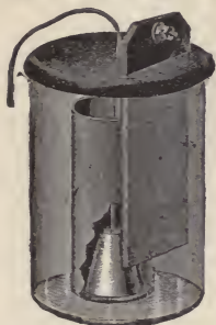
FIG. 64. FULLER BICHROMATE CELL.
