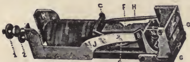
FIG. 131. COMBINED JACK AND SELF-RESTORING DROP. A JACK, JK LINE SPRINGS, B CONTACT FOR SLEEVE OF PLUG, F CONTACT FOR TIP OF PLUG, N OPENING OF JACK, ENTERING WHICH PLUG RESTORES DROP SHUTTER E , I LINE DROP COIL, D SPRING NORMALLY IN CONTACT WITH J , WHICH CUTS OUT COIL WHEN PLUG IS INSERTED BREAKING CONTACT BETWEEN J AND D , H ARMATURE PIVOTED AT C . DROP E ENGAGES WITH TIP OF H WHEN DROP IS IN NORMAL POSITION. 1 AND 2 ARE BINDING SCREWS FOR HOLDING JACK AND DROP IN POSITION ON THE FRAMEWORK OF THE BOARD.
