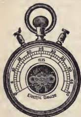
FIG. 99. BATTERY GAUGE (SCALE READINGS HAVE NO DEFINITE VALUE; COMPARISON MUST BE MADE WITH CELL OF KNOWN STRENGTH).
