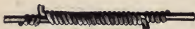
FIG. 83. BRITANNIA JOINT. wire or bound to it by a piece of tie wire. A piece of the end is generally left projecting beyond the joint for attaching the leading in wire; with the twisted sleeves the leading in wire can be joined directly to the line.
