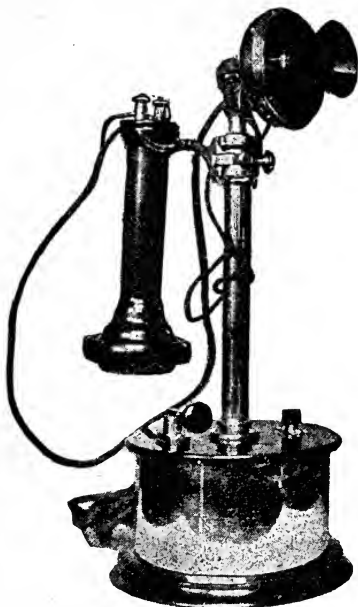
FIG. 40. SOLID BACK TRANSMITTER ON DESK SET.
