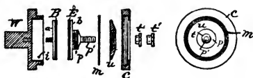
FIG. 42. DETAILS OF SOLID BACK TRANSMITTER. W ELECTRODE CHAMBER, i INSULATING LINING, B BACK ELECTRODE. a BRASS BACKING, E FRONT ELECTRODE, b BRASS BACKING, p THREAD FOR NUT U , m MICA WASHER, u NUT FOR CLAMPING m IN PLACE, p' THREAD FOR t AND t , c COVER OF W , TT NUTS FOR CLAMPING FRONT ELECTRODE TO DIAPHRAGM
