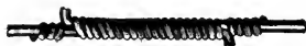
FIG. 83. BRITANNIA JOINT. A piece of the end is generally left projecting beyond the joint for attaching the leading in wire; with the twisted sleeves the leading in wire can be joined directly to the line.
