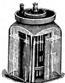
FIG. 61 A. TYPE OF AGGLOMERATE LE-CLANCHÉ CELLS.
