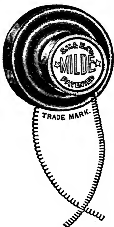
FIG. 130. THE MILDE TRANSMITTER. REAR VIEW OF CHAMBER, SHOWING WEIGHT ON BACK ELECTRODE.
