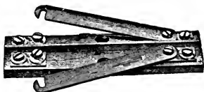
FIG. 93 A. SNEAK CURRENT PROTECTOR. OPERATES BY HEATING OF SMALL COIL, WHICH CAUSES FUSIBLE WIRE TO MELT.
