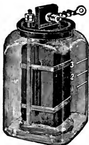
FIG. 61. AGGLOMERATE OR "PRISM" FORM OF LE-CLANCHÉ CELL.
