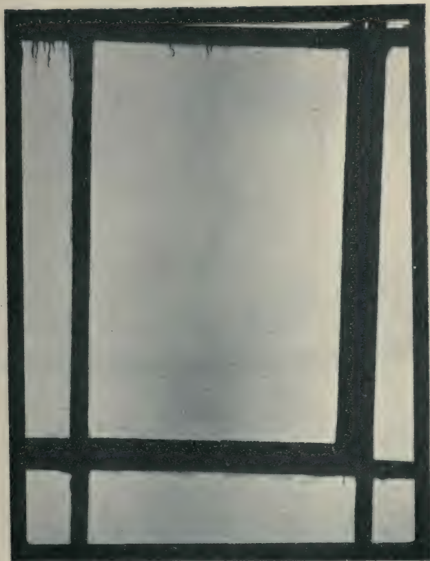
PLATE 11.—WINDOW.—Taken under the same conditions as Plate 10, but with the camera back vertical. Here the inner frame is wider at the top than at the bottom.
