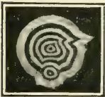
FIG. 156.—Effect of Flaws in Objective.
