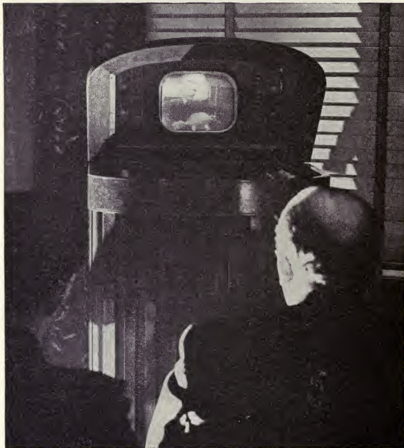
ZENITH REFLECTING RECEIVER, 12-INCH TUBE
