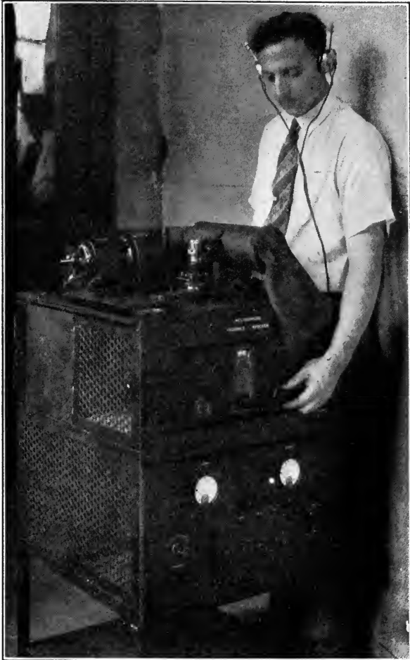
FIG. 71.—Westinghouse facsimile receiver. Note photographic dark bag over cylinder on which print is made.
