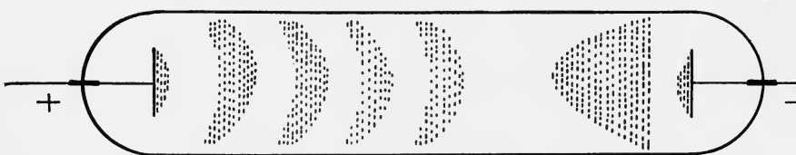
FIG. 33.—When a certain stage of rarefaction is reached in a discharge tube the glow breaks up into striations.
