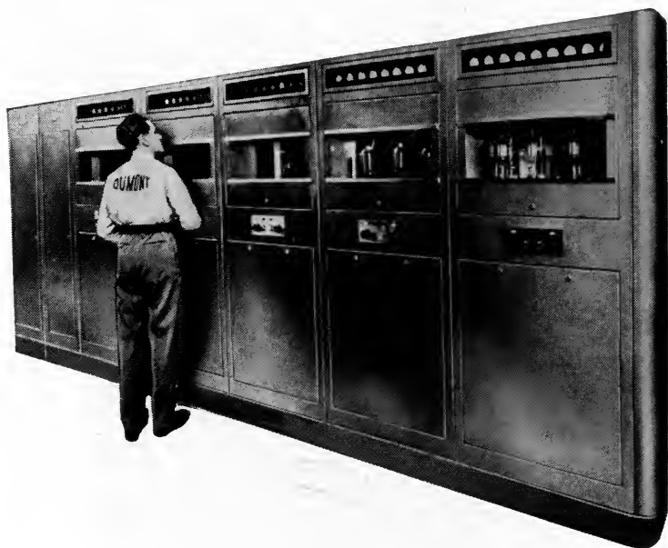
FIG. 18.—WABD transmitter at 515 Madison Ave., New York City. ( Allen B. DuMont Laboratories, Inc. )
