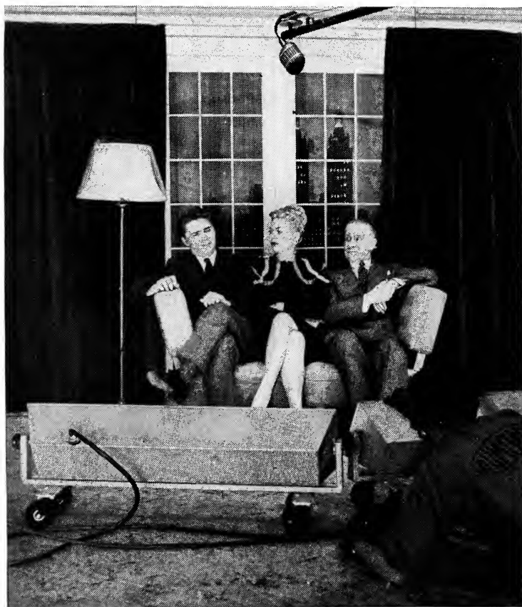
FIG. 41.—Mobile incandescent floor lights at WABD. ( Allen B. DuMont Laboratories, Inc. )
