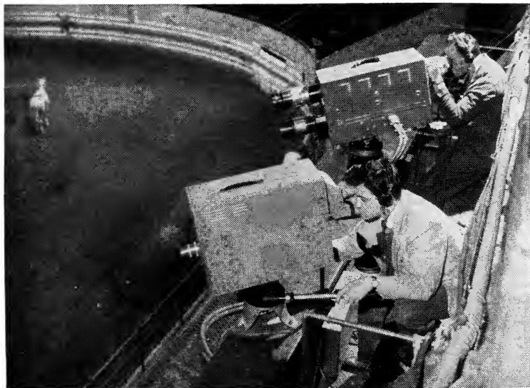
FIG. 102.—Scenes from Madison Square Garden are picked up by RCA's new supersensitive television camera (foreground) and by a conventional camera to demonstrate the advantage of the new development in providing greater depth of perception and clearer views under imperfect lighting conditions. ( Radio Corporation of America. )
