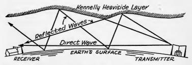
Pursuing the "wave" idiom, this is a crude presentation of the fashion in which radio frequency impulses travel from transmitter to receiving stations. The loss of power in transit is sometimes called "fading," and is believed to occur from absorption of the electrons by the earth and atmosphere.
