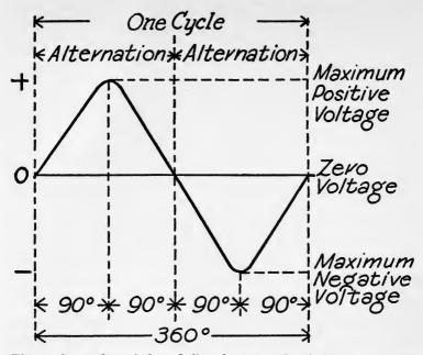
This is the mathematical symbolism for one cycle of alternation in the performance of electrical current. Vertically, it measures the units of voltage per cycle, horizontally, the units of time. Out of this graphic representation has grown the myth that electricity moves in waves, with "short waves" (greater numbers of cycles per second) and "long waves" (lesser numbers).
