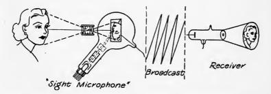
As in sound, so in sight broadcasting. The difference here is that modulation occurs upon the light-sensitive plate and is converted back into the shadow of substance by propulsion of electrons upon fluorescing material at the broad end of the receiving valve. May we be forgiven the phrase, "sight microphone"?
