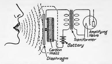
When one speaks before the microphone the sound waves strike against a diaphragm, agitate the carbon mass behind it, and cause current to flow through the microphone in amounts varying according to the frequency of the sound wave.
