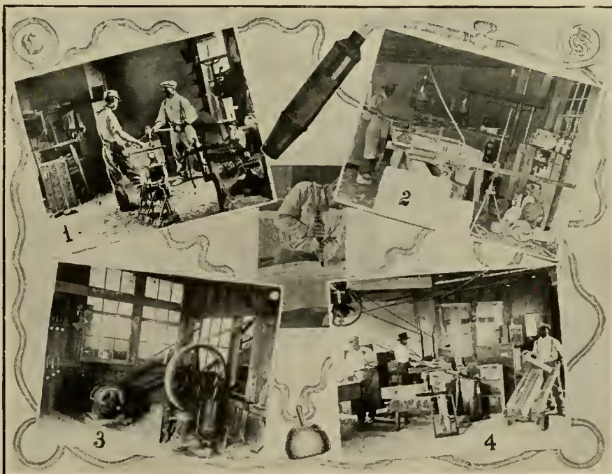
1 Blacksmith Shop 3 Electric Dynamo and Air Compressor where the Power is Generated 2 Granite Polishing Shed for Pneumatic Tools 4 Boxing Department
