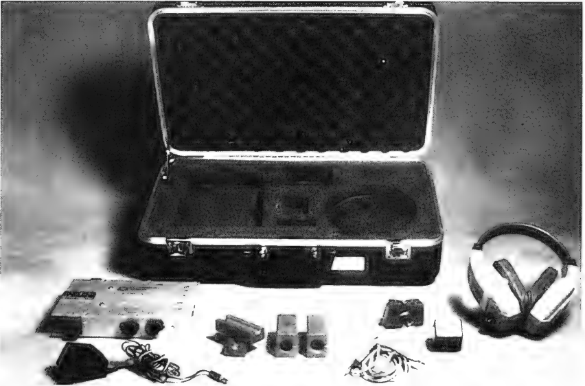
Figure 2. MT 75 wire rope inspection device.
