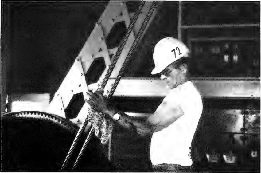
Figure 9. Inspector using the “rag and visual” inspection method.
