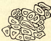
FIG. 20. Cross section of jute fibres.
