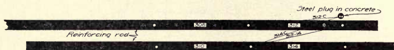
FIG. 61. ARRANGEMENT OF GAUGE LINES TO TEST FOR MOVEMENT OF BAR RELATIVE TO CONCRETE.
