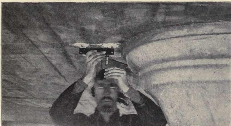
FIG. 13. ORIGINAL BERRY EXTENSOMETER IN USE.
