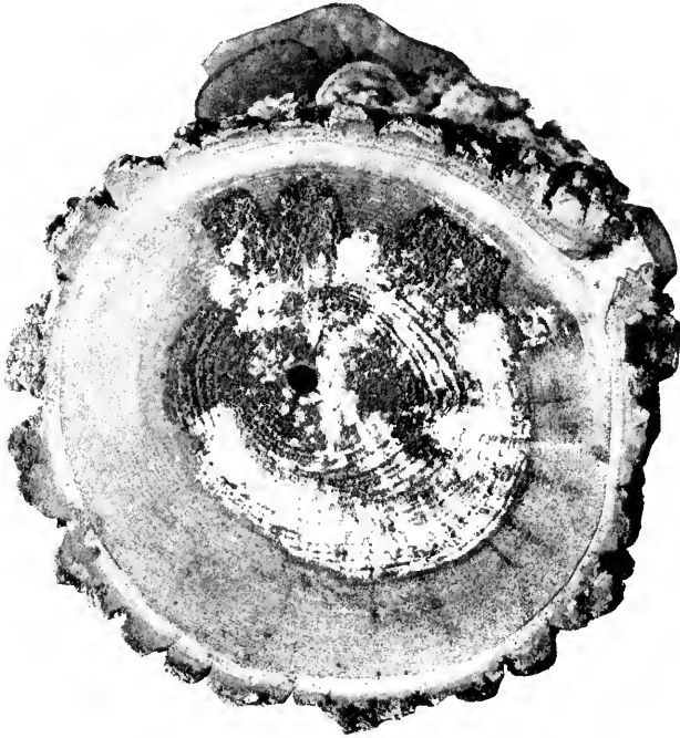
FIG. 262. Cross section of a stem of white ash in which a saprophytic fungus has destroyed a part of the heartwood. The obvious mycelium pictured on the cut surface grew after the section was removed from the tree and placed in a moist chamber. From U. S. Department of Agriculture.
