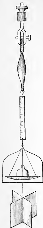
FIG. 178. — Du Bois-Rey- mond's apparatus for the study of elastic ex- tension in muscle (after Rosenthal). The gradu- ated rod attached to muscle is to be observed with a lens.
