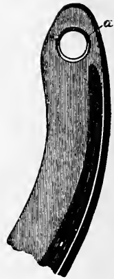
Ground-surface of the end of a branch of shoe, showing (a) hole and counter-sinking for a screw-calk (one-half natural size).
