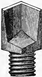
Corner calk (Winkelstollen) of Branscheid & Philippi.
