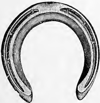
Right front shoe with concave ground-surface (“convex iron”) to prevent “forging.”
