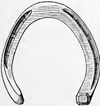
Shoe with interfering branch, interfering shoe (ground-surface).
