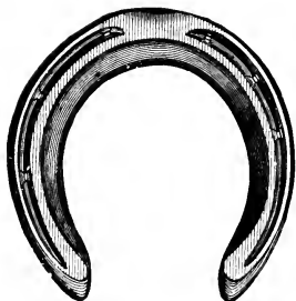
Right front shoe with concave ground-surface ("convex iron") to prevent "forging."
