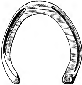
Left hind shoe with interfering branch (ground surface), for base-narrow standing position.
