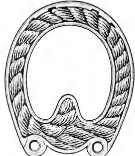
The same with beak-formed bar.
