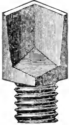
Corner calk (Winkelstollen) of Branscheid & Philippi.
