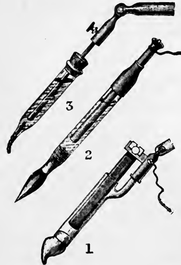
FIG. 335.—NON-POLARIZABLE ELECTRODES. 1. Du Bois-Reymond's. 2. Von Fleischl's. 3. d'Arsonval's.
