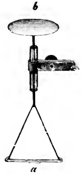
FIG. 91.—Apparatus for determining the blood pressure in the capillaries, after Ludwig. The small glass plate a is placed on the skin, and the pan b is loaded with weights until the skin underneath a is blanched.
