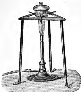
FIG. 23.—Heating Magnesium in Air.
