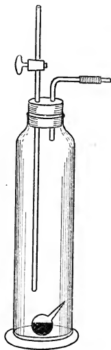
FIG. 204. — Experiment to show Solubility of Hydrobromic Acid in Water.
