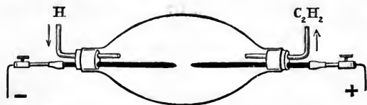
FIG. 334.—Berthelot's Synthesis of Acetylene.
