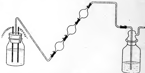
FIG. 134.—Filling Glass Bulbs with a Mixture of Chlorine and Hydrogen.
