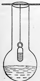
FIG. 310.—Conversion of White into Red Phosphorus.
