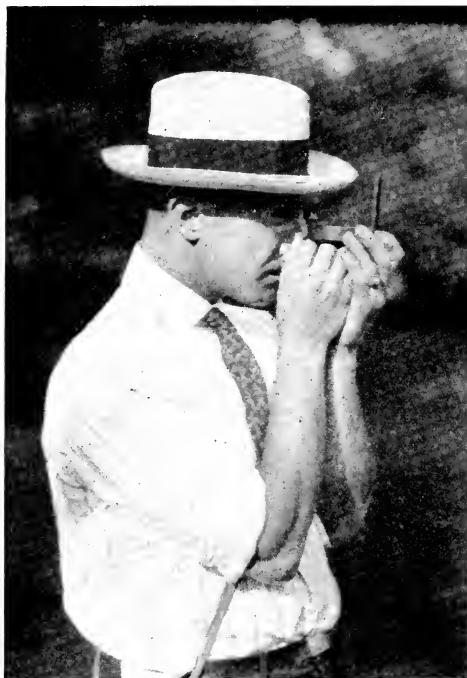
FIG. 16. USING THE PRISMATIC COMPASS
