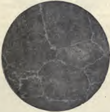
FIG. 57.—Crystalline structure of annealed cementite-pearlite steel (hypereutectoid steel). Photomicrograph by H. T. Manuel. Magnification 265 times.
