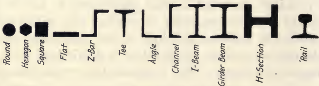
FIG. 48.—Common rolled sections.
