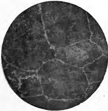
FIG. 57.—Crystalline structure of annealed cementite-pearlite steel (hypereutectoid steel). Photomicrograph by H. T. Manuel. Magnification 265 times.
