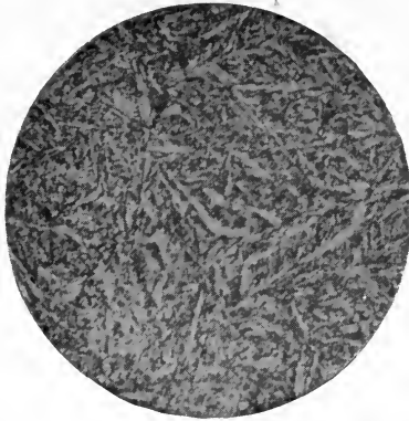
FIG. 58.—Martensite, characteristic crystalline structure of very suddenly cooled hypereutectoid steel. Photomicrograph by H. T. Manuel, Univ. of Illinois. Magnification 265 times.
