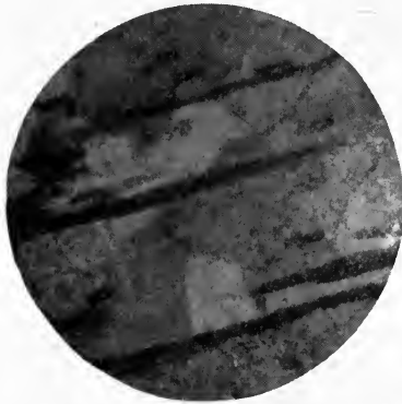
FIG. 30.—Longitudinal section of wrought iron showing slag "fiber." Photomicrograph by E. O. Dixon and Jos. Simons. Magnification 350 times.
