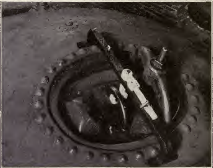
FIG. 73.—Method of locking with government seal the top of a tank containing condemned products.
