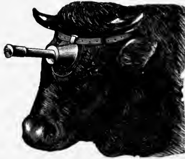
FIG. 13.—Head of bull with shooting apparatus, attached, according to Staehl-Stoff.
