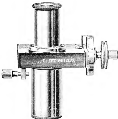
FIG. 207.—Screw micrometer eyepiece (Filar micrometer).
