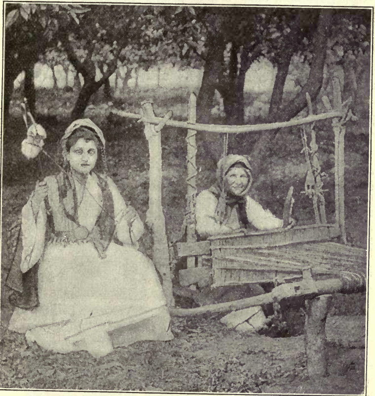
FIG. 18. — PRIMITIVE WEAVING AND SPINNING. SPINDLE AND DISTAFF. LOOM WITH HEDDLE.
