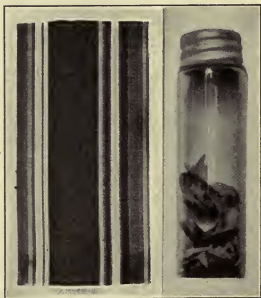
FIG. 137. — WEIGHTING OF SILK. THE BOTTLE CONTAINS THE MINERAL WEIGHTING LEFT AFTER BURNING A PIECE OF SILK LIKE THE SAMPLE SHOWN.
