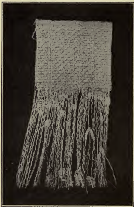
FIG. 136. — MIXED LINEN AND COTTON TOWELING TREATED WITH SULPHURIC ACID. THE LINEN REMAINS IN THE FRINGE.
