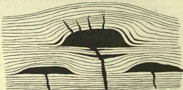
Fig. 308.—Ideal section of three "Laccolites," after Gilbert.
