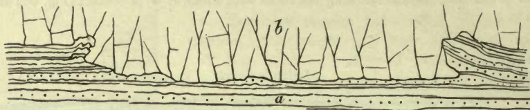
Fig. 304.—Section at base of south front of Salisbury Crags, showing portion of strata cut out by intrusive diabase. a , sandstones, shales, &c.; b , diabase. Length of section, 22 feet.
