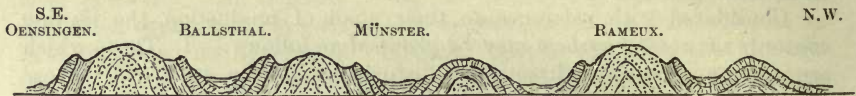
Fig. 500.—Symmetrical Flexures of Swiss Jura (the ridges coinciding with anticlines and the valleys with synclines).
