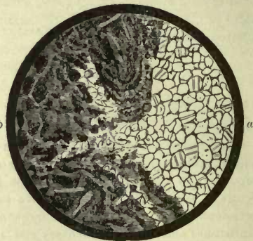
Fig. 342.—Section of limestone (a) (Burdie House) converted into granular marble by basalt (b). Magnified 20 diameters.
