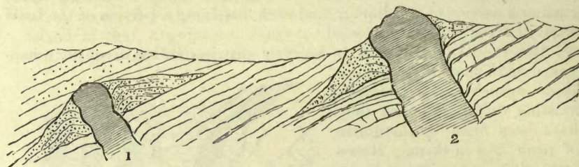
Fig. 323.—Diagram-section to show the structure of old volcanic vents, and how they may be concealed and exposed.
