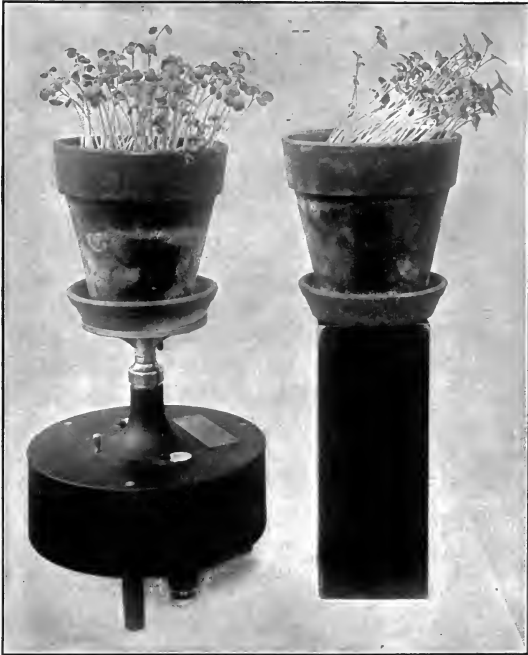
FIG. 75.—Sets of Radishes grown side by side in a chamber lighted wholly from the right hand side; but those on the instrument were kept continually revolving.
