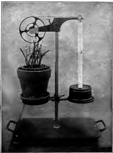
FIG. 121.—An auxograph, or recording growth measurer, in action. Its construction is explained in the text. Unfortunately the record, in the form of a spiral line on the cylinder, does not show in the picture.
