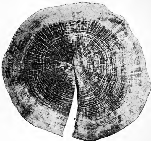
FIG. 26.—Photograph of the transverse section of a log of oak, about one sixth natural size. The cortex and bark are removed, and the outline is bounded by the cambium. The pith appears as a mere dot in the center; the medullary rays radiate from this, and the annual rings (about forty in number) are arranged concentrically around it. A large crack has formed along the plane of a medullary ray as the section dried. (Müller.)
