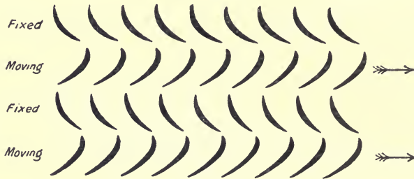
FIG. 99.—Arrangement of blading for Parsons turbine.
