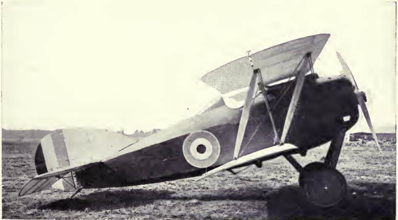
FIG. 117.—'Vickers 16 D' Scout, fitted with 200 h.p. Hispano Engine.
