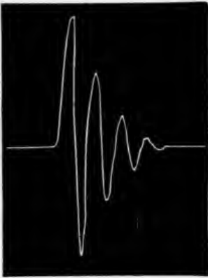
FIG. 73. Tracing of the oscillations in a mercurial manometer. The first upward stroke is due to sudden rise of pressure. The subsequent fall below zero and the other oscillations are due to the inertia of the mercury, and not to any external force. Compare with Fig. 53.
