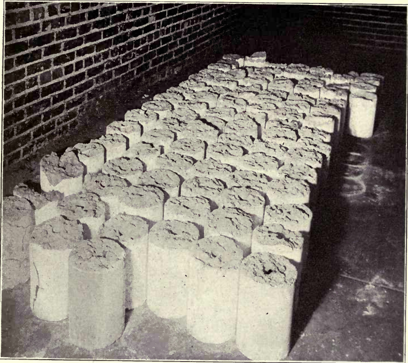
FIG. 6. GENERAL VIEW OF BROKEN TEST CYLINDERS
