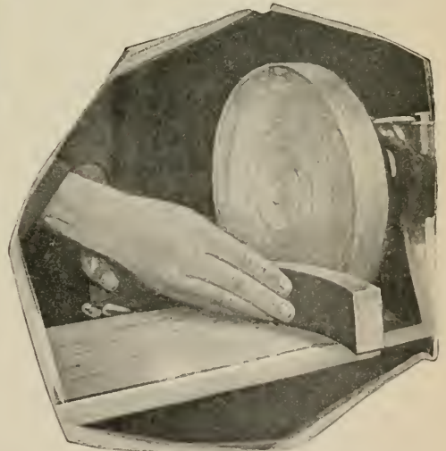
FIG. 70.—How pieces such as the segments of the apron under a circular table top are sanded.
