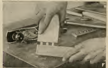
FIG. 26.—How to make doweled butt joints. Gaging and marking for the dowel holes, boring them, making the dowels, and testing the joint.
