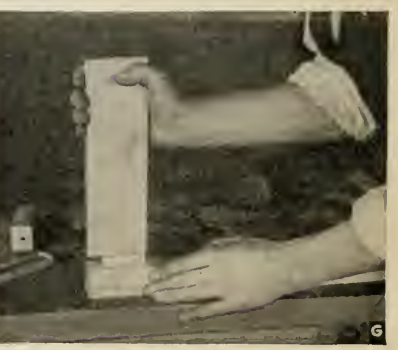
FIG. 28.—Steps in making a mortise and tenon joint. How to gage and mark the mortise and tenon in the leg and rail of a table; using the auger bit and chisel to make the mortise, and the rip saw to cut the tenon; pressing the finished joint together.
