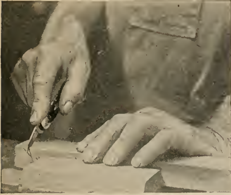
FIG. 4.—The shoulder of a tenon can be cut more easily if a notch is first made for starting the saw.
