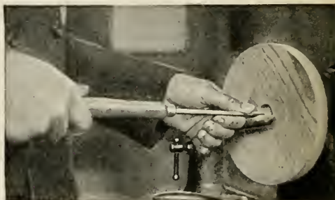
FIG. 47.—Upper view: Using the toe of a keen \frac{1}{4} -in. skew chisel to bore the hole that is to take the tenon of the candlestick upright. Lower view: Marking the diameter of the base with dividers held on the T-rest and centered by trial.
