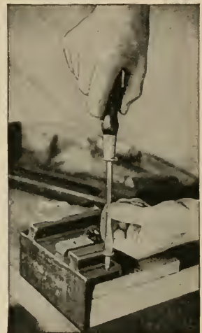
FIG. 5 (at left).—A homemade wooden stop for planing. FIG. 6 (center).—Fastening an iron stop in place. FIG. 7 (at right).—How a rapid-acting vise is fitted. The same vise is shown in use in Fig. 1.
