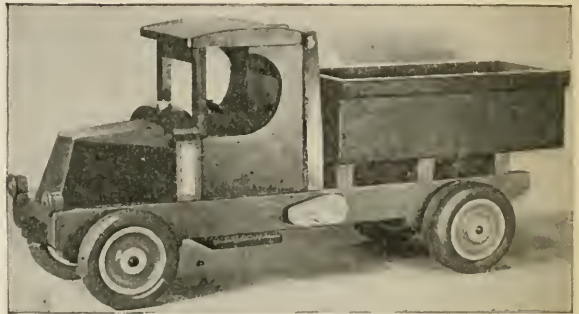
FIG. 8.—The dump truck has a foolproof elevating mechanism, the parts being a dowel, a spool, and a piece of tape.
