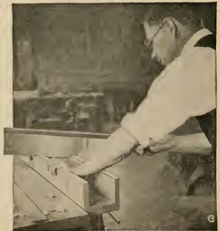
FIG. 19.—Steps in making a miter box of wood. The work must be done with extreme care, and the cuts should be made with the saw which is to be used with the box.
