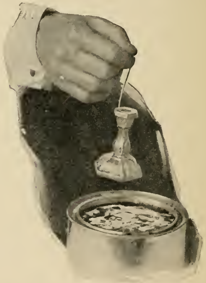
FIG. 10.—Candlestick with marbled finish obtained by drawing it through a film of floating colors.
