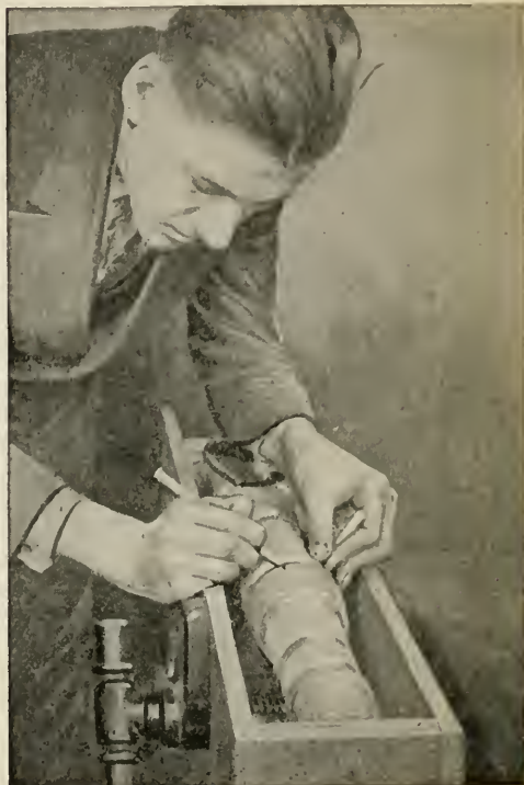
FIG. 66.—Marking a column to be reeded. The divisions are transferred from a paper strip.
