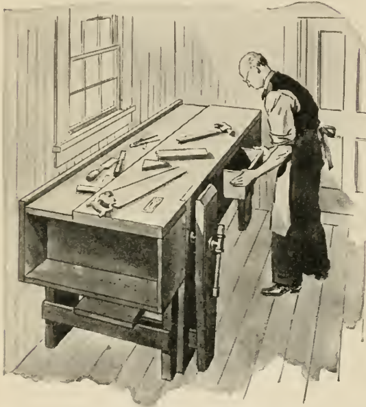
FIG. 17.—A man-size bench of the carpenter's type for the amateur mechanic who does much woodworking and repairing.
