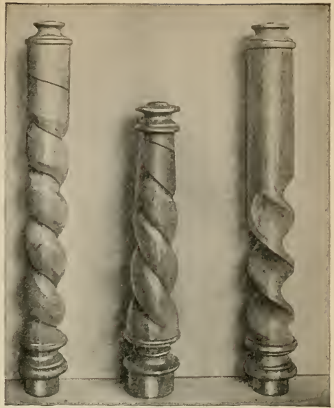
FIG. 72.—Single spiral turning (at left); tapered double spiral (center); hollow spiral (at right).
