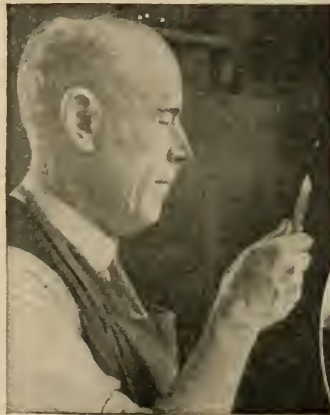
FIG. 9 (at left).—Scrutinizing the cutting edge to note the width of the white line.
