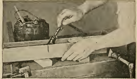
FIG. 20.—Hot glue always should be applied freely to both edges of the wood to be joined.
