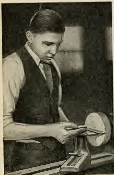
FIG. 46.—After the base has been trued with a round-nosed chisel and smoothed with a square-nosed tool, it should be tested for flatness.
