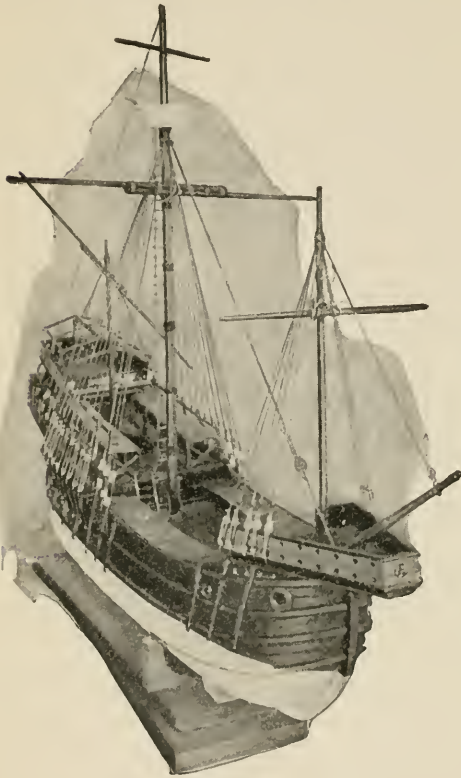
FIG. 35.—The model partly rigged and with masts, shrouds, yards, main- and forestay in place.
