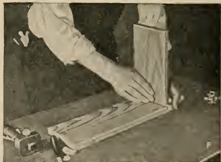
FIG. 30.—Steps in making a dado joint. Marking the inner cut for the dado and the width of the stock; making a V-groove for starting the saw; sawing to the gage lines, removing the waste wood with a chisel, and testing the joint.
