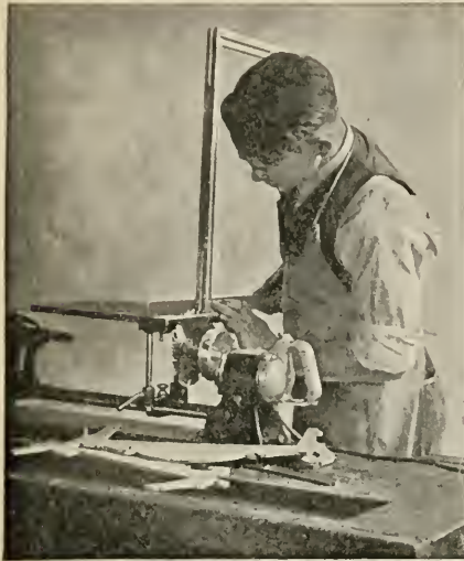
FIG. 26.—The grooves for the head and bottom pieces are cut after the frame is assembled and cleaned.
