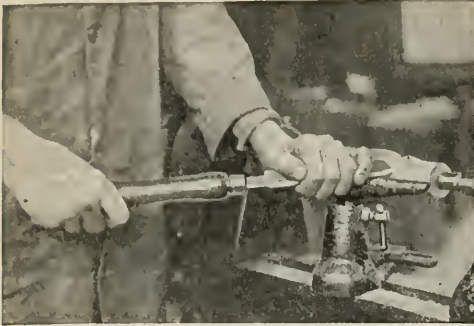
FIG. 17.—Start the cut near the dead center and move the tool toward it. Hold the tool as illustrated and stand in the position shown.
