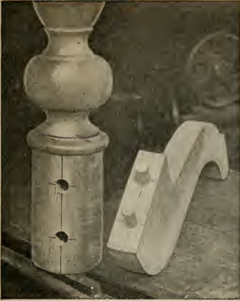
FIG. 33.—One of the legs with dowels inserted, all ready to be glued to the turned column.
