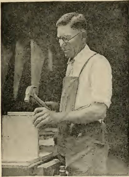
FIG. 7.—Whenever wood must be hammered, use a soft block of waste wood as a protective cushion.
