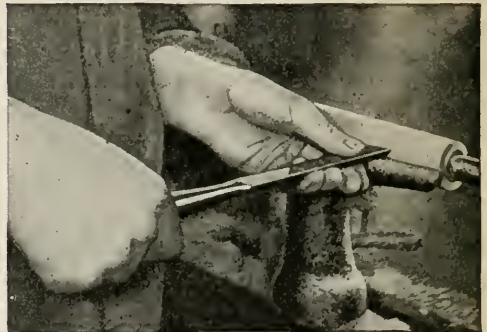
FIG. 19.—Smooth the cylinder with a square-nose turning chisel or a firmer chisel with a long blade.
