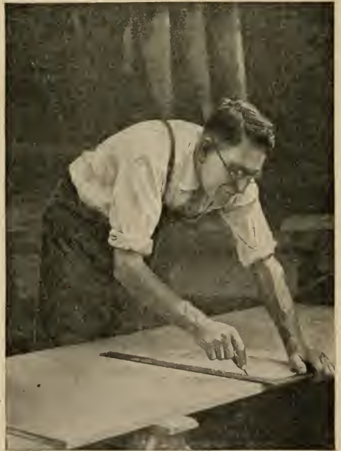
FIG. 1.—Scribing a line along the inner edge of a steel framing square.
