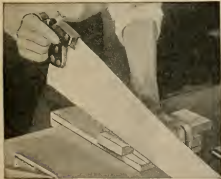
FIG. 27.—Rabbeted joints. How to measure and mark the width and depth of the rabbet, saw out the surplus wood, and nail the boards together.
