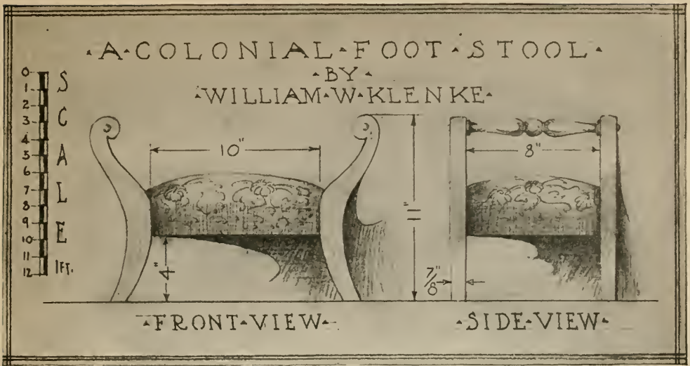
FIG. 2.—Original pencil sketch of the footstool, which was made as a preliminary to illustrating the various steps in machining the parts. For details, see the drawings in Fig. 3.
