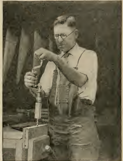
FIG. 6.—Boring a dowel hole with a block of wood on the bit to serve as an improvised depth gage.
