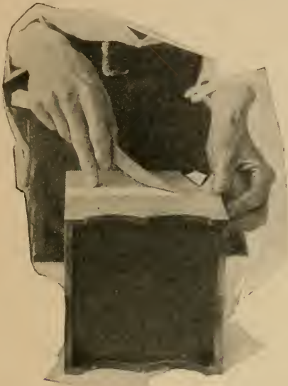
FIG. 6.—After it has protected one part while another is being painted, the masking tape is peeled off.
