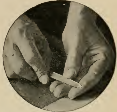
FIG. 46.—How the point of a file is ground for drilling glass.
