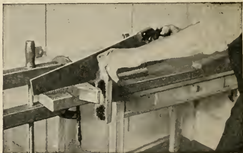
FIG. 4.—This method of attaching the hand screws is a useful one when boards are to be ripped.
