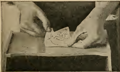
FIG. 14.—A center line on the back of the transfer is a great aid in placing it centrally and vertically.
