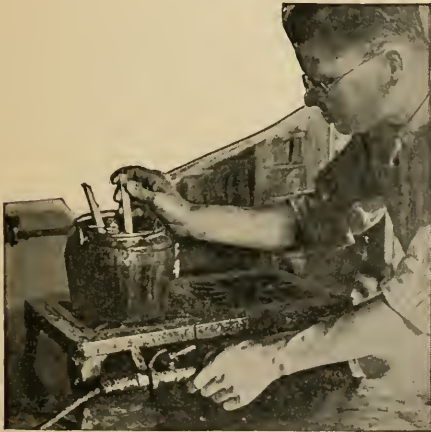
FIG. 19.—A dairy thermometer may be used to avoid accidentally heating animal glue beyond 150^{\circ} F.
