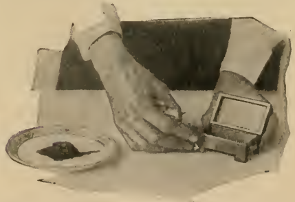
FIG. 8.—Dusting gold bronzing powder on a jewel box previously coated with japan gold size.
