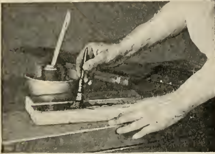
FIG. 21.—Liquid glue should be brushed on vigorously and all parts of the joint well covered.
