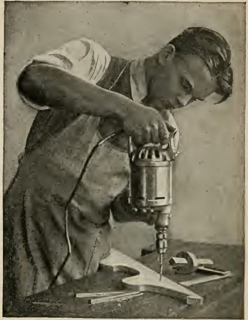
FIG. 33.—Some types of portable jig saw motors can be easily dismantled and used as electric hand drills for drilling screw holes, making holes for inserting a jig saw, and other light work.
