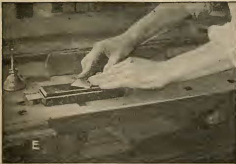
FIG. 1.—Steps in sharpening chisels, plane irons, and other chisel-edged cutters. How the keenness of the edge may be tested on the thumb nail.
