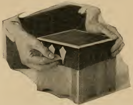
FIG. 7.—Gummied tape is used to make masks for shielding certain parts of the design before painting.
