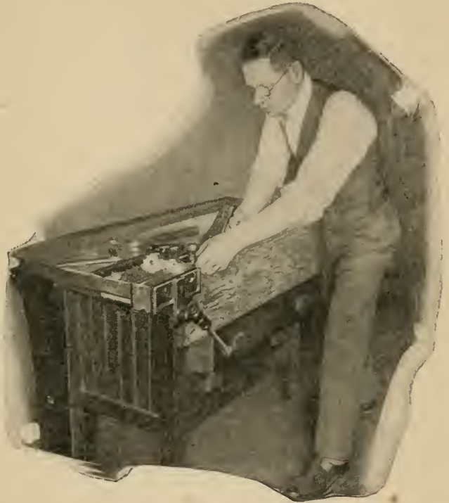
FIG. 10.—Planing at the small cabinet bench. Note how a drawer has been partly drawn out to help support the long board.
