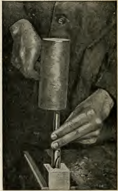
FIG. 6.—Use a wooden mallet to drive the live center into the wood. This is particularly important when the stock is hard wood.
