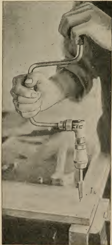
FIG. 17.—Using a brace and bit makes easy work of driving a screw.
