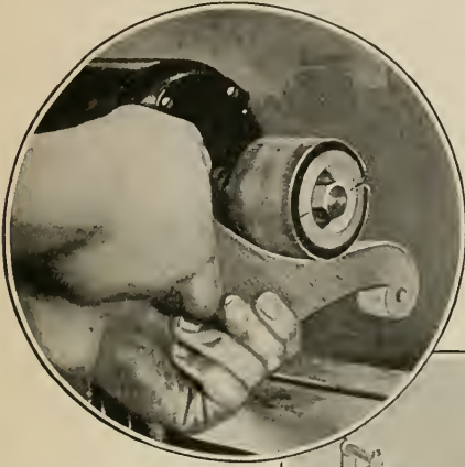
FIG. 7 (above).—Cleaning up the convex curves of the legs on a drum sander. If this type of sander is not available, a sanding cylinder can be turned from wood for use in the lathe. The edges of the sandpaper should be wedged into a longitudinal groove by means of a small strip of wood. FIG. 8 (at right).—The spindles or handles in the lathe. Calipers are used to make measurements.
