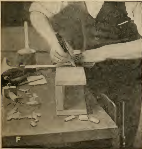
FIG. 19.—Steps in making a miter box of wood. The work must be done with extreme care, and the cuts should be made with the saw which is to be used with the box.
