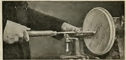
FIG. 45.—Making the base circular by removing wood from the edge with the toe of a skew chisel. Note the position of the T-rest.
