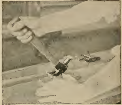
FIG. 11.—A block under the claws of the hammer is necessary in drawing long nails.
