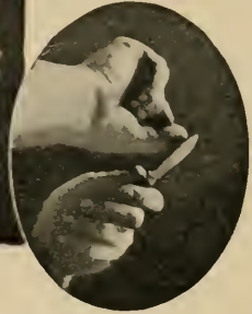
FIG. 10 (below).—The thumb-nail method of testing sharpness.
