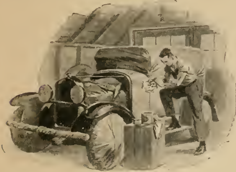
FIG. 1.—Cover the motor, wheels, and top with paper or old clothes before applying the paint remover.
