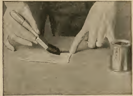
FIG. 15.—Varnish or other adhesive is applied to the transfer and allowed to stand until "tacky."
