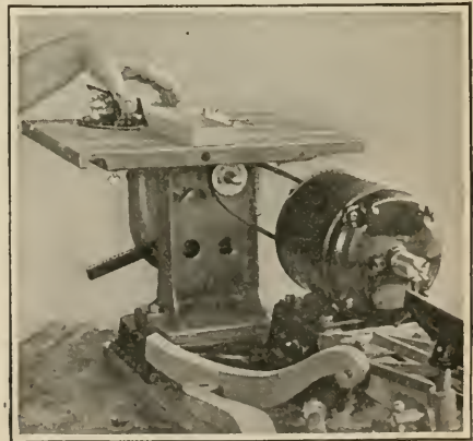
FIG. 4.—How to hold the rails (sidepieces) when cutting them to exact length on the circular saw.
