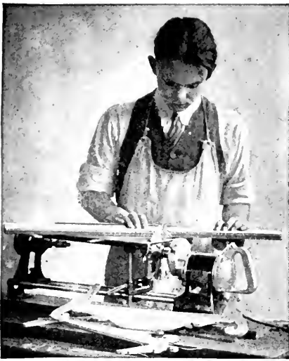
FIG. 23.—The common method of cutting miters with the cut-off fence at 45 degrees and the table level.
