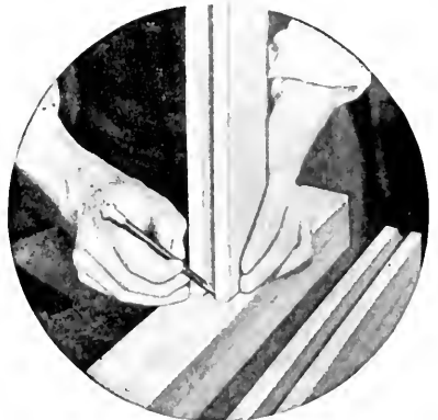
FIG. 14.—Mark the legs by placing the end of each rail in position.
