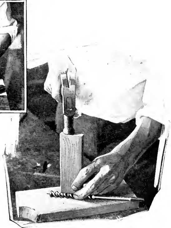
FIG. 6.—Doctoring the screw point with an oilstone (usually called a "slip") that has a thin edge.
