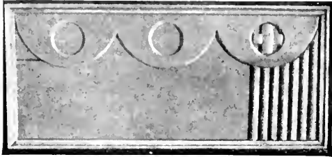
FIG. 19.—An unfinished mantel ornament, showing how the apparently carved parts are glued on.
