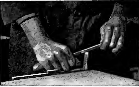
FIG. 4.—The edges of scraping tools are sometimes turned over with a burnisher to form a burr or almost microscopic hook.
