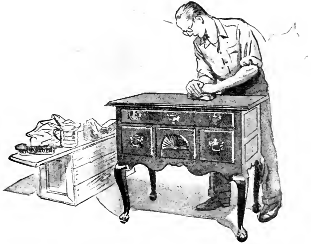
FIG. 24.—The final polish is given to the oiled and waxed top of a low boy with a rubbing block.
