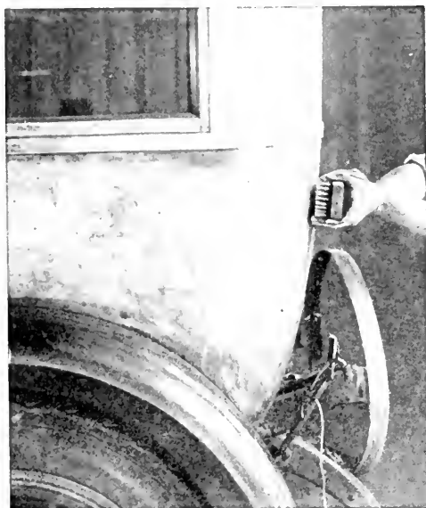
FIG. 3.—Thoroughly clean the body of all old paint by "scratch brushing" it with a stiff wire brush.
