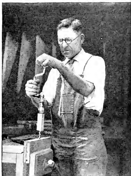
FIG. 6.—Boring a dowel hole with a block of wood on the bit to serve as an improvised depth gage.
