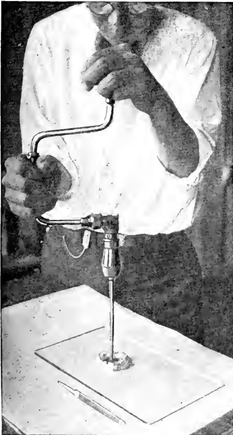
FIG. 45.—The way a file is held in a brace for drilling glass. Note the ring of putty which retains the turpentine.
