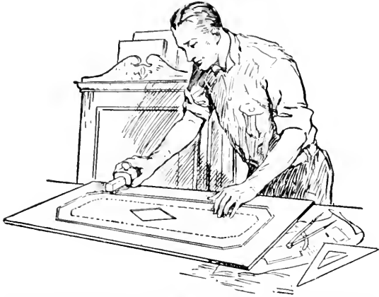
FIG. 33.—Cutting grooves for inlays with a modified marking gage which has a cutter instead of a point.
