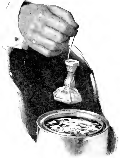
FIG. 10.—Candlestick with marbled finish obtained by drawing it through a film of floating colors.
