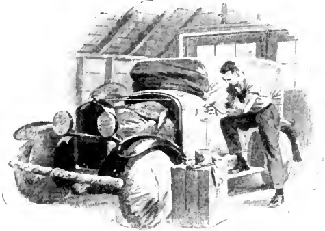
FIG. 1.—Cover the motor, wheels, and top with paper or old clothes before applying the paint remover.
