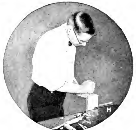
FIG. 31 How to make a multiple dovetail joint of the type used in drawers. This is often called a "lapped" dovetail because the joint does not show from the front. It is one of the strongest and most craftsmanlike joints.
