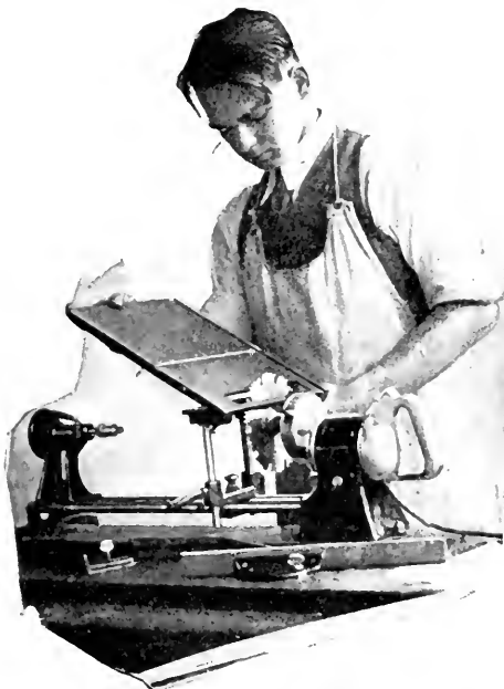
FIG. 24.—Cutting miters by tilting the table at 45 degrees and placing the molding on its edge.
