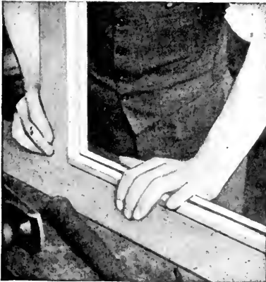
FIG. 15.—Strips are nailed to the legs to correspond to the grooves in the rails.
