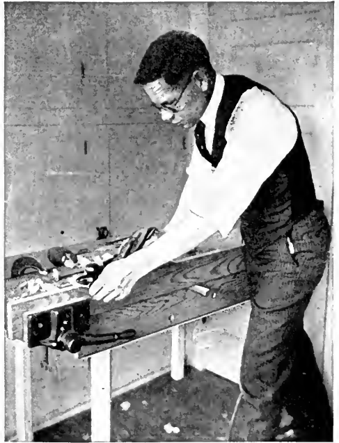
FIG. 1.—Bench top with quick-acting woodworking vise for use on a kitchen table. The top is fastened on the table with heavy C-clamps.
