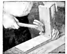
FIG. 8 (left).—Handling a hammer for straight nailing. Note that it is gripped near the end.
