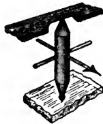
THE DOUBLE PIVOTED NEEDLE OF PEREGRINUS.
