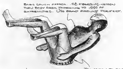
TRANSITION TO CAPSULE 100 FIBERGLAS-NESTON. FIBERS LAY TANGENT TO BASIC COUCH.
