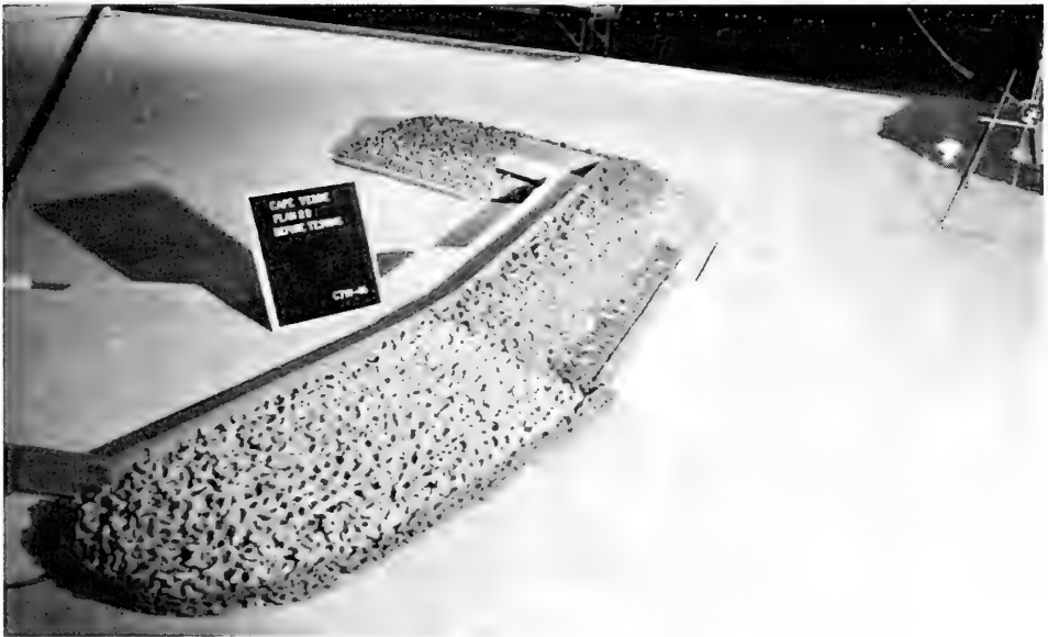
Photo A44. View from north of plan 2D breakwater trunk before testing
