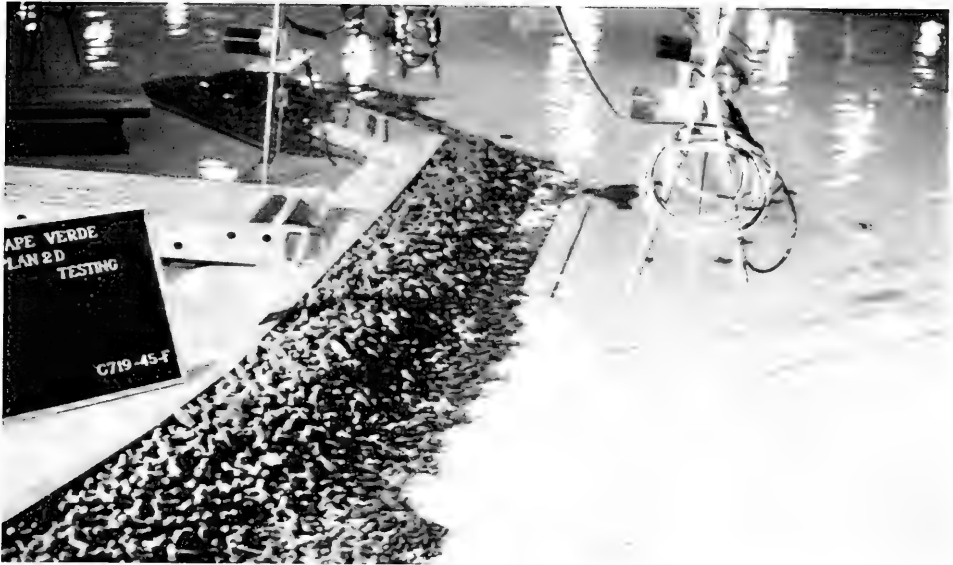
Photo A45. View from north of plan 2D breakwater trunk after testing with total sequence
