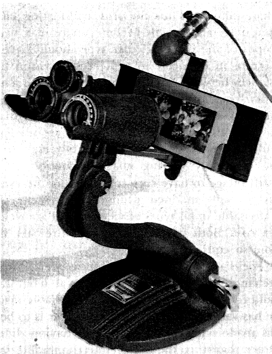
Fig. 3-5. Telebinocular. One of the most satisfactory of the Brewster type viewers. This is the instrument used in the laboratories of the Stereo Guild for all stereograms of abnormal separation, such as the old "parlor" type of view.
