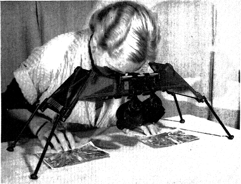
Fig. 3-6. The Ryker, a small version of the Wheatstone stereoscope used for viewing prints up to six inches square, is an aerial photo type of viewer. Courtesy J. P. Medders.
